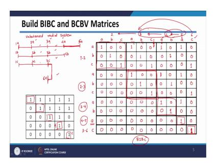
Now, let us see how we can use this for unbalance system. So in case of unbalance system; so, for unbalanced radial system so, here we are not considering till now weekly may system. So, in case of unbalance radial system, let consider this unbalanced radial system let us say this is your branches between 1 and 2, then between 2 and 3, 3 and 4, 4 and 5 and then there is 6 here.
