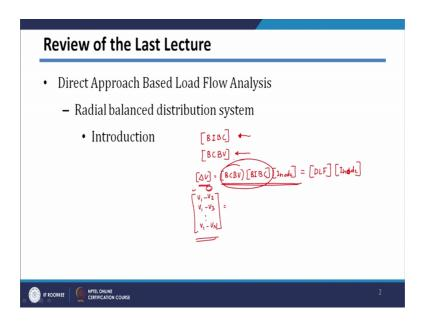
And we have seen that you can actually form two matrices which we call it as actually BIBC matrix, which is Bus Injunction to Branch Current matrix, which converts your bus injunction to directly into branch current.
