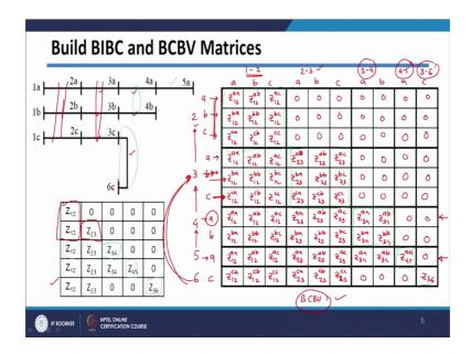
So, this how we can build your BIBC matrix. Let us see how we can build your BCBV matrix. So, BCBV matrix for 3 phase system. So, in this case we have seen that here that there will be bus numbers 2 3 4 5 and 6 and, here there will be branch number so, there is branch between 1 and 2, 2 and 3, 3 and 4, 4 and 5 and then there is 3 and 6.
