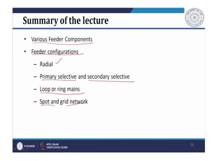
So, in this particular lecture we have seen various components of your feeder. Then we have seen feeder configurations, those configurations are basically radial configuration, primary selective and secondary selective configuration, loop and ring mains configuration and then spot and grid network.
