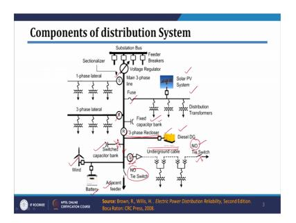
So, if you see this particular figure I have shown various components of distribution feeder.
