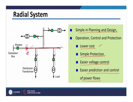
Now, we will see various feeder configurations. So, first commonly used feeder configuration is radial system. So, in this figure I have shown it so, there will be actually feeder mainline which is going and then laterals will be connected to this main feeder.
