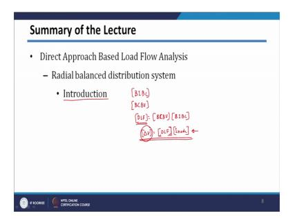
So, in this particular lecture we have seen direct base approach based load flow analysis. We have seen the introduction and introduction, we have seen that we if you form this matrix, which is called as BIBC matrix, which basically converts your bus injection to branch currents and then another matrix, which is BCBV matrix which basically converts your branch current to bus voltages.
