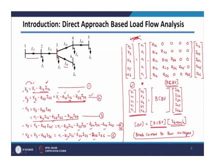
Now, let us consider one more matrix which we can write which is called as a BCBV let us see how we can write it. So, we know that your voltage V 2 is actually equal to voltage V 1 minus Z 1 2 into I 1 2 this is basically this drop which is Z 1 2 multiplied by I 12.
