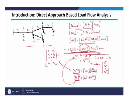
So, basically we have got two equations one is called I branch is equal to you may write BIBC matrix, which con convert branch injection to bus injection to branch current multiplied by your I node. And one more equation we got that is delta V voltage difference will be equal to your BCBV matrix multiplied by your branch currents. So, basically your BCBV matrix convert your branch current to bus voltages.
