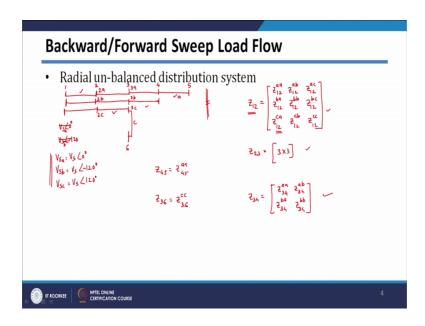
So, you are having see this three phases n and say this is bus number 1, this is bus number 2, and then same three phases are extended till bus number say 3. So, here your bus number 3 and after bus number 3 say only 2 phases are extended, third phase is
