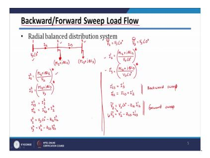
Let see how it works? So, in this case you are having say simple 2 base system; like this then there are 2 loads are connected say this load is PL 2 plus j QL 2 and this loads say PL 3 plus jQ L 3. And, this is bus number 2 bus number 3 and this is your bus number one source bus, the voltage at this bus is given and will remain constant on all iteration. So, we are keeping the bus of this voltage at this bus one will be constant at say V S angle 0 degree.
