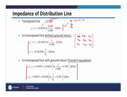
So, we have seen in case of transpose lined your equation for the impedance is this one, where this is nothing but just j omega 2 into 10 raised to minus 7, which is converted into kilometers. So, it should be the multiplied by multiplied by 1000.
