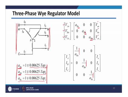
After, transformer we have gone for three-phase regulator model. And we have seen that a regulator model your depends upon your tap ratio, and the transformation of voltage will be decided by your regulator setting. And, this regulator setting is given by one minus plus 0.00625 into Tap of a a Rb. So, setting of b or ratio of b will be given by one minus plus 0.00625 to Tap of b similarly you can get for third.
