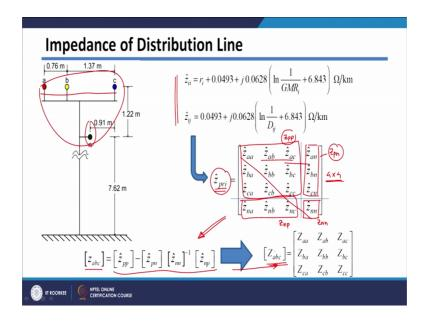
So, if there are 4 number of conductors into system the primitive impedance matrix will be 4 by 4, which will be having entries like this there will be 4 conductor corresponding
