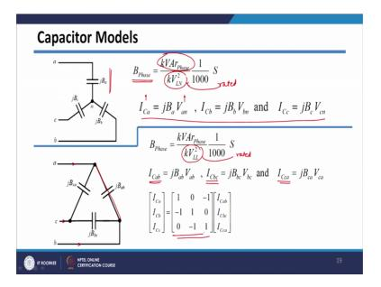
So, so, susceptance we of the capacitor bank or capacitor in phase will be calculated based on rating of that capacitor. And, line to neutral rated voltage. So, this is actually I should say rated voltage. And, once you get the susceptance then we can get the currents in various phases, and delta connected also similar thing will happen only thing is here we have to use line to line rated voltage of the phase because this capacitor getting connected, between line to line.
