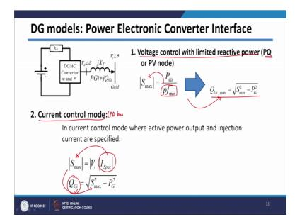
And then finally, we have seen DG models for photonic based converter interface. So, in this case there are again 2 modes of operation one is actually voltage control or reactive power mode limited reactive power mode and then current control mode. So, in this basically the current is control to this specific value from that current we have seen that we can calculate maximum apparent power it can supply, and from this maximum apparent power we can get what will be the Q G i of the generator.
