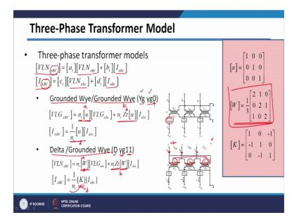
And, then we have gone for three-phase transformer. So, in case of three-phase transformer also we have derived the a b c d parameters of those transformer. So, in this case also we have writ10 primary voltages and currents in terms of secondary voltages and currents. So, these are the primary side voltages to represent added by capital abc.
