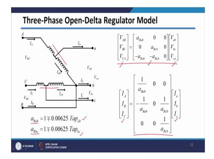
We also seen if there is open delta regulator so, many time to say one regulator we can use open delta, because output three-phase voltage can only be can be controlled by only using only 2 regulator. So, in that case it is used as open delta regulator and these 2 regulators can be used control three-phase voltages at output. So, in that case also we have derived.
