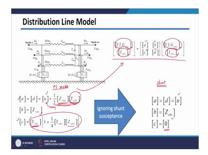
And, then lines can be modeled as pi model or short line model. So, if you are modeling as a pi model, we have seen that your equations for pi model are like this where u is unit matrix. So, of 3 by 3 size and this is your impedance matrix, which I have got this is our admittance matrix, here also this is admittance and impedance matrices.
