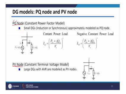
As PQ node or PY node where P and Q specified and from that your injected current will be calculated. However, in case of PV node your power is specified and voltage of that node is kept constant.
