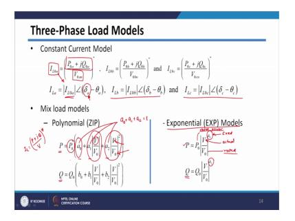
In case of constant model that is next model here first you have to get the rated current value. So, that rated current value will be calculated based on rated power, which is this divided by rated voltage. So, from the rated voltage and rated power first get rated current.
