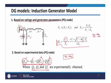
Then in case of induction generator model we have seen 2 models one is based on parameter. So, from the parameters of the generators, we can get of this reactive power absorbed by generator that is QGi including the power factor correcting capacitor.
