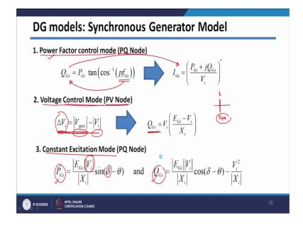
And, then we have seen synchronous generator model we have seen 3 types of model one is when the power factor is controlled, when voltage is controlled and then third is excitation control. And, we have seen that when whenever we are using power factor control mode you have to use PQ node PQ node always considered as negative load applied at that particular bus. So, it will act as a your generator will act as a negative load.
