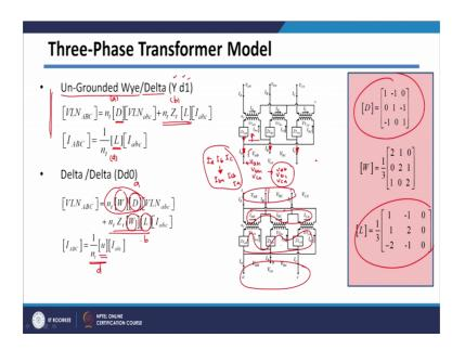
Then, we have seen third configuration that is ungrounded Wye to delta configuration is called as Y d 1 configuration. So, primary Y connected which is ungrounded. So, g is not written here then this is delta and one there is 30 degree phase shift.
