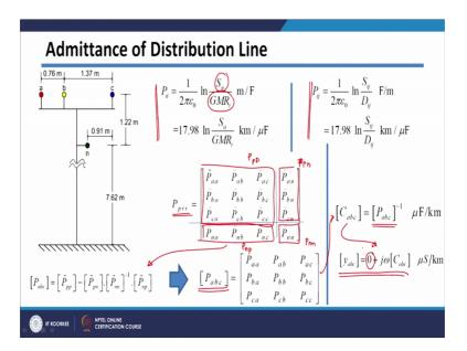
So, phase similar to phase impedance matrix we can get phase impedance matrix by using the potential coefficient. And, the expression which you derived for potential coefficients are like this which again depends upon various distances and your GMRS of the conductor. So, by knowing the GMRS and distance with respect to image, we can get this potential coefficients and potential coefficient matrix will also be number of conductor by number of conductor soil.
