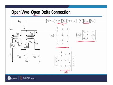
And, then we have seen one model with open wye and open delta connection also this also you have seen that which can pref we can prefer it because it saves you one transformer here. So, from only 2 transformer you can give three-phase supplier to any
