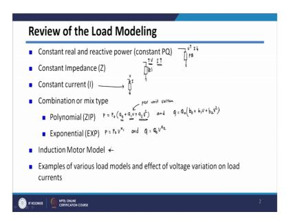
Constant impedance model, constant current models; we have seen that these models we have considered different type of this model, because they behave differently with respect to applied voltage. Means if you see this constant real and reactive power model, if the voltage across this increases, it will draw a less current to keep power constant.
