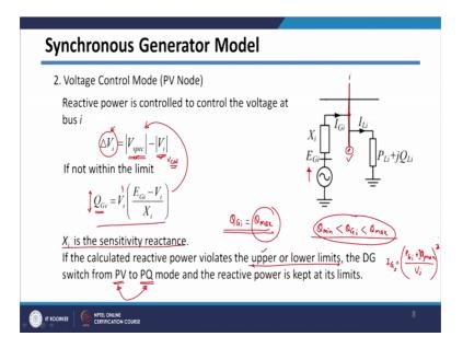
Means we can actually control the voltage of this particular bus to specified a value and this specified value.
