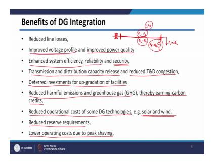
So, this is basically happening because you are connected some relative load at load end. So, here this is PL plus jQL which is load is connected at the end and if you are connecting some DG here, which is generating PG plus jQG then real power flowing from this one be PL minus PG and reactive power will be QL minus QG.
