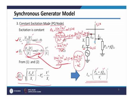
So, whenever the voltage at this bus is changing your reactive power generated by this generator will change. So, since excitation is constant you can keep this EG constant here and whenever this is change in their terminal voltage, there will be change in the reactive power supplied with generator
