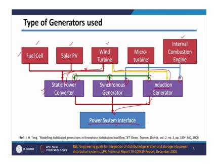
So, we need some kind of power electronic converter here to convert it into AC which can be connected to power grid or distribution grid. In case of wind turbine there are 2 types is one is variable speed and one is constant speed. So, in case of variable ts speed DGs we use basically a DFIG with some kind of power tonic interface.
