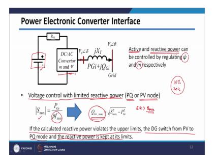
Now, let us see how we can model if some sources which are interfaced with power electronic based converters. So, here basically in case of fuel cell or in case of solar protocol type or in case of battery which can be represented here. So, this is DC source which is may be renewal solars like solar PV or fuel cell and it will be then there will be DC to AC converter, and this will be the voltage at this bus will be AC voltage.
