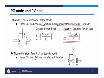
Generally in case of small DGs maybe it is synchronous or induction generator it is approximately modeled as PQ node. So, in case of PQ node, we model them as a negative loads. So, if you see this diagram here this DG is connected at I th bus the load at this I th bus is say QLi PLi plus jQL qLi and generation at this bus is PGi plus j QGi the current which is generated by DG is fed through the fed to the grid and the current taken by the load is shown by iLis.
