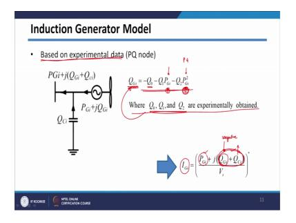
Another method of modeling induction generator is basically experimental based. So, many times the data is not available. So, we can modeled by model through experimental data. Experimental data is will be modified like this means it is getting from the reactive power is basically depend on the real power and as well as real power square, and there will be a some relation between this real power which is having some part, which is
