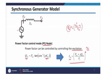
We start with first synchronous generator; synchronous generator can be modeled as simple like this you are having generator, this is generated voltage beyond the synchronous beyond before the synchronous reactance and this is nothing, but your terminal voltage. And this synchronous generators can be run into three types of modes; one is called as a power factor control mode, where the power factor of this DG will be controlled to some value some constant value may be.
