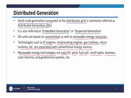
So, this is generally small scale generation connected to the distribution grid. So, generation which is connected to distribution grid, we call it as a distributed generation. Now these are basically a small generators connected over the or spread over your distribution area, and it is commonly known as distributor generation. So, small scale generation connected to distribution grid is referred as a distributed generation.
