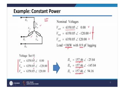
So, in this case I have taken this example of load which is connected in star fashion and the nominal voltages means rated voltages of this load since I am considering say eleven Kv system. So, per price voltage will be eleven by root 3. So, basically they are in volts and loads in all the three-phases I am considering same load that is 1 megavolt of load is connected in all the three-phases; means each phases I am taking 1 megavolt of load and the power factor of this load is say 0.9.
