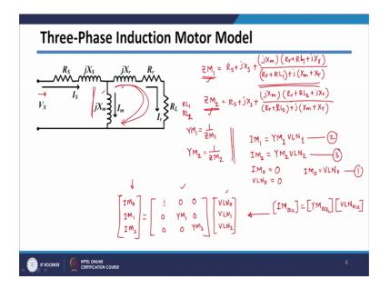
So based on that, I will get equivalent positive sequence network equivalent of this one; so ZM 1 is nothing but positive sequence when I am considering R L 1 resistance here. So, equivalent impedance of this circuit ZM 1 will be equal to R s plus j X s plus there will be this parallel branch.
