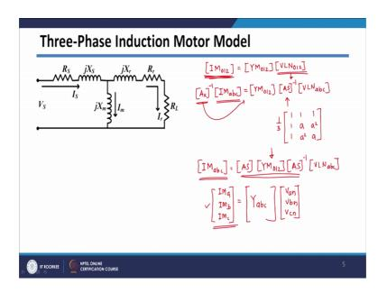
So, in this case, we have got IM 0 1 2 which is equal to YM 0 1 2 into VLN 0 1 2. Now, we know that there is sequence conversion matrix which is basically if you multiply this matrix by As inverse or we can say this is equivalent to As inverse multiplied by IM abc. So, if you want to convert phase quantities into sequence component, we know that we
