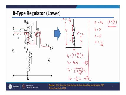
Opposite of this, when your switch is connected to L position, your current path will be something like this. So, in this case current will be coming like this through this winding with regulatory winding, it will go 2 terminal L ok.
