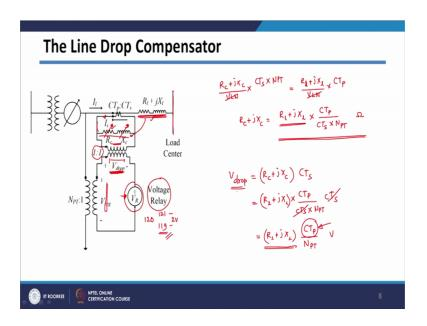
So, in this case we have got R C plus j X C divided by VLN into C TS into your N PT which is equal to R L plus j X L divided by your VLN multiplied by your CT primary ratio.
