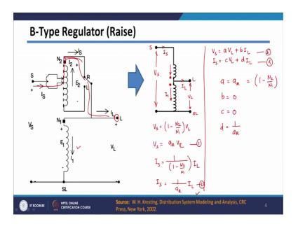
And in the last class we have seen the operation also of A type as well as B type of regulator and what we are seen depending upon your position of yours this reversing switch R or L, we have seen various configurations. So, in this case when your switch is on R position, then the current will flow like this. So, I S will go and then I S will come from this side and then it will from it will get added to your I 1. So, in this case if you see, this dot is connect get is towards your L point.
