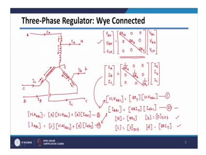
So, I am just taking your B type regulators which are connecting in. So, it will be having 2 winding. So, this is a phase A; one is one winding is this. This basically winding is regulator winding and then one winding is your common winding or series shunt winding. Then similarly, we can plot another phase. We will also having 2 windings and then, there will be third phase. So, this is regulating winding and this is your shunt or common winding.
