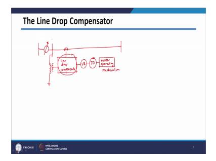
So, in this case say this is your feeder and your interested the control the voltages at the far end of the feeder and then say to control the voltage of this particular bus, you are connecting regulator here and then, here actually the voltage which is given and to control the regulator positions, we use this line drop compensator circuit.
