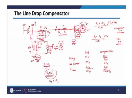
Across this current transformer, some impedance will be connected and then there will be 1 transformer which is having ratio 1 has to 1. So, your having this transformer which is having ratio 1 has to 1 and then you are having this voltage transformer here and then this signal is actually connected to your voltage relay circuit. So, basically this signal is coming from your voltage transformer.
