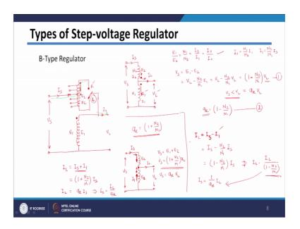
Now, let us see B type regulator. The construction is similar. However, only the connections are different in this case also there are two types of winding; one is again we need regulator winding with tap positions.
