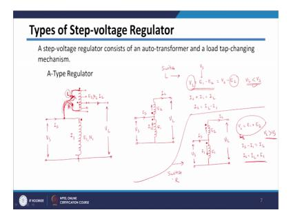
So, in case of type A regulator you are having this circuit here something like this. So, as I told you it is auto transformer which are basically it two windings; one is called as common winding and one is called as regulator winding. So, these are two windings. So, basically this is your regulating winding where we need to use taps.
