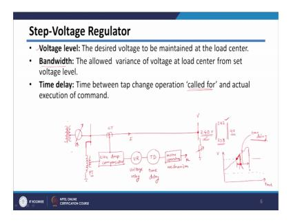
So, if this say the your feeder end, this is start of the feeder and which is basically connected by say regulator and say there is transformer here and we want to regulated the voltages at this, once function of this one we want to regulate at this ok.
