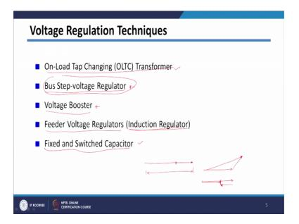
So, one important voltage regulated component is actually your On-Load Tap Changing Transformer. So, we know that then generally your taps will be provided on high voltage side of your transformer and by increasing and decreasing the taps, we can change the voltage at the secondary side and depending upon the voltage requirement at other end of the feeder, we can increase or decrease the tap and regulate the voltage at secondary end.
