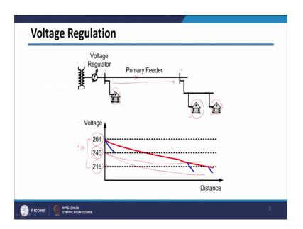
So, whenever there is no load condition if these loads are not there you can see that voltage both the points will be same. However, whenever there is loading on your feeder, there will be current which is fluent through the feeder and which will basically there will be drop across the feeder. So, voltage which is reaching at consumers which are connected at the far end will experience lower voltages.
