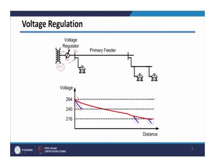
So, if the voltage of the second this side of the transformer say 240, then by using voltage regulator I can make the voltage at the secondary end of the regulator say 264 which you have shown it here. Even though, there is drop across the feeder, we can bring the voltage within the limit ok.
