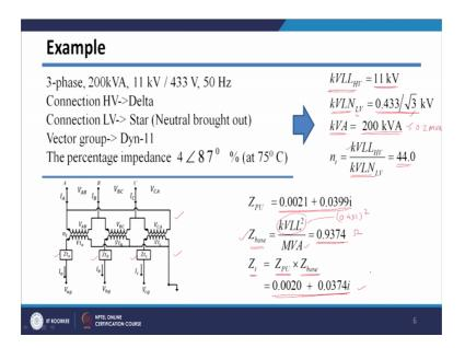
So, for turns ratio, we need to know, because on a primary side, it is delta. So, across the winding, there will be line to line voltage, and secondary side is star connected, so across the one winding, the voltage will be line to neutral voltage.
