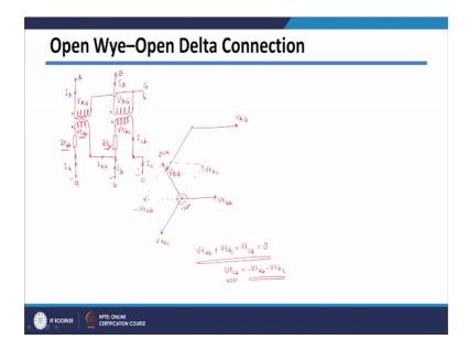
So, in this case we as I told you we are going to use only two transformers. So, let us say, these are the two transformers here. And then I am taking the impedances on secondary side, so these are the impedances.
