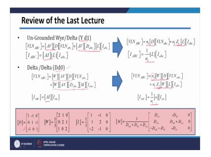
In the last lecture, we have derived for two different transformer, those are actually ungrounded wye by delta connection, so this particular vector group is Y d and 1. And for that connection you have got A parameter, which is A multiplied by D, where this D matrix is done by this one, which basically convert your line to neutral voltages to line to line voltages. And then your b parameter is, A V multiplied by Z t abc multiplied by L. And your D matrix is, A I multiply by L.
