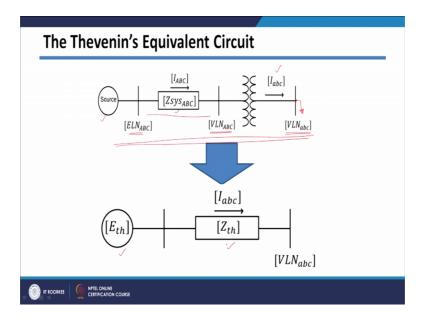
Now, see many times in basically short circuit calculation. We need to know, Thevenin's equivalent circuit at that particular short circuit point. Say in this case, what I shown is there is source here, then this bus voltage is V L N A B C, I am E L N A B C I am calling. And then say there is a transmission line, which is having impedance matrix also a Z system A B C. So, 3 by 3 matrix of your transmission line
