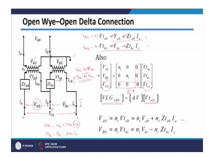
Let us see, how can we derive, the abcd parameters for this particular matrix here, this particular transformer here. So, in this case, again I am taking that transformer on primary side, which is basically we connected open wye, because third transformer will not there. In this case, secondary is delta connected open delta, because third transformer will not there, which is basically makes you delta closed.
