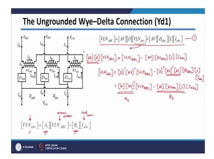
We have also calculated a capital A parameter and capital B parameter and these capital A and capital B parameters I have defined at like this; which are basically used to calculate line to neutral voltages on secondary side in terms of primary side voltages and the load currents. So, generally load currents are known primary voltages are known because those are applied voltages. Then load terminal voltages will be calculated using this capital A parameter and capital B parameter.
