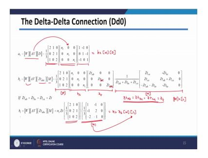
So, if I take these parameters on next slide. So your, a t parameter we have seen it is W multiplied by multiplied AV by D. Out of this AV can be represented by diagonal entries of n t and this those can be taken it out. So, this can be written as n t multiplied by your W matrix multiplied by your D matrix because this term I can take common out.
