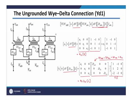
So, let us simplify it. So, we have got this a and this is your b. So, a is AV multiplied by D, AV we have seen it is diagonal entries n t and D matrix is given by this expression. So, in short form I can write, from this I can take n t common out. So, it will just remaining unit matrix, unit matrix multiplied by some matrix will be it will be same.
