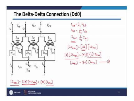
So, this is how we can get a parameter and b parameter, to get c and d parameter we have to take the current relations into account. So, in this case I can write I AB will be equal to 1 by n t into I ba. I BC will be equal to 1 by n t into I cb, I CA will be equal to 1 by n t into I ac and if you write them in short form.
