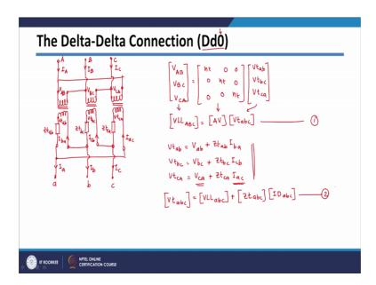
So, we have seen ungrounded wye by delta connection. Now, let us see your last connection that is delta delta connection and in this case I am considering vector group which is Dd 0 means, place displacement between primary and secondary quantities will be 0. So, they will be connected like this. So, you are having this transformer 1, transformer 2, and this is transformer 3. The impedances are referred on secondary side so I should represent them here and these are the terminals.
