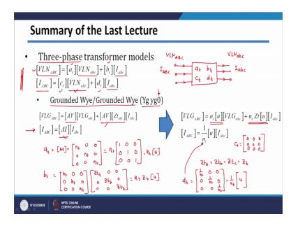
Then we have seen this grounded wye by grounded wye connection in the last class. Before that we have seen modeling of three phase transformers and we have seen that three phase transformers can be modelled using a b c d parameters, to are those are represented as a t b t c t d t. These are your secondary terminals of the transformer, these are your primary terminals of the transformer. Here the voltages are V capital ABC.
