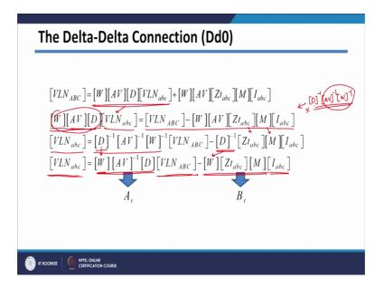
So, if you do this so, this term I am taking on left hand side; so here I, taken this and the remaining terms on right hand side which are basically this. Now, we want to eliminate this term here because on left hand side we want only VLN abc here. So, what we can do? We can multiply this whole expression by D inverse. So, whole expression will be multiplied with D inverse multiplied by AV inverse, multiplied by your W inverse.
