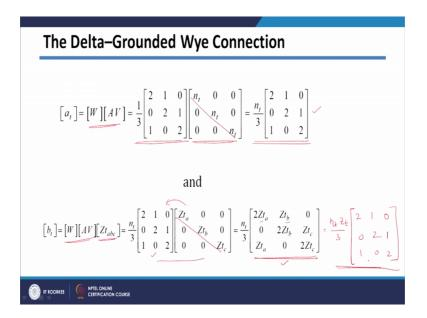
So, we have got a t which is equal to W multiplied by AV, W matrix we know which is this one and AV matrix is a transformation matrix which is n t which is diagonal matrix. So, we can easily write n t these are diagonal which will get multiplied to each of the entry basically it will come out of the matrix. So, it will be n t by 3 and to this particular matrix.
