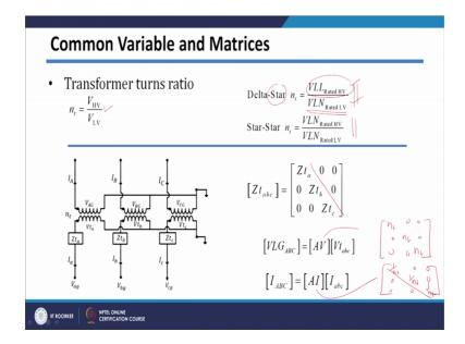
Before that I will just revise the terminology turns ratio we are going to see it is voltage on primary side or generally in case of distribution it will be HV side. So, voltage on primary side divided by rated voltage on secondary side. So, for different configuration depending upon phase voltage means voltage across the winding you have to see while calculate turns ratio.
