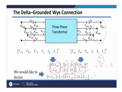
For various connections we want to get abcd parameters. So, we have calculated abcd parameter for single phase connection to winding transformer where abcd parameters are just one number. However, since if you observe these are actually three phase voltages which are three voltages, this also three voltages there are three currents on primary side and secondary side.
