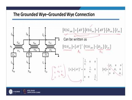
So, we are got this equation here and we want actually write this equation secondary side voltage in terms of primary side voltage and secondary. So, we can take this on left hand side. So, in that case if you take this on right hand side and then if you multiply everywhere by AV inverse, in this case it will become VLG abc secondary side voltage in terms of primary side voltage and secondary current. So, so we have got in required format.
