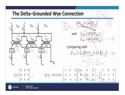
Let us see how we can get currents. So, in this case first we will take currents which are winding currents. So, as we know that winding currents are related by turns ratio. So, on this side winding current is I a. So, the current which is flowing through the secondary winding is I a and I b and I c.
