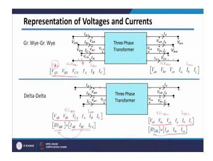
So, V AG represent way phase to ground voltage and if in case of ungrounded neutral. So, if this neutral is grounded neutral terminal available it is grounded then I will say V AG and if it is ungrounded means in this grounding is not there then I will say V AN voltage with respect to neutral terminal.
