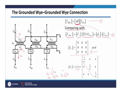
So, these are a t and b t parameter; let us see how we can get c parameter and d parameter; c parameter and d parameter we can get it from current equations. We have seen current transformation equation that is the current which is flowing in primary side and current which is flowing in secondary side; in this case current which is flowing in primary side is I A and current which is flowing in secondary side is a opposite direction it is small I a ok.
