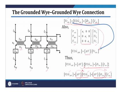
So, basically we have got this Vt abc which I explained is basically line to ground voltages of these terminals that is V ag V bg and V cg which is basically in this particular matrix. And all the three terminal voltages those are V ta V tb and V tc which are in this Vt abc matrix, this is impedance matrix and line current matrix we have derived in last slide.
