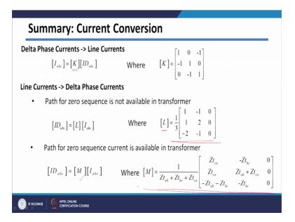
And in case of current convergent to convert delta phase currents to line currents we have got this K matrix and to convert line currents to delta phase currents we have got this L matrix. However, there are two cases because depending upon zero sequence current path is available or not we need to use L or M alternatively. So, whenever there is
