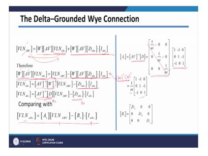
So, we want to make this load side voltages in terms of source side voltages and so, will just write that way by taking this on left hand side and this on right hand side. So, if you
