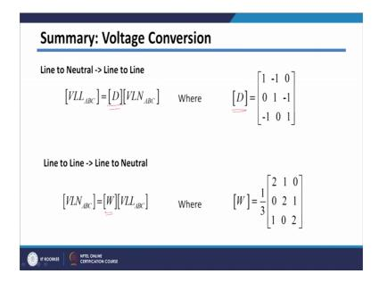
So, for transforming line to neutral voltage to line to line voltage we have got D matrix, then to convert line to line voltages to line to neutral voltages we have got this W matrix.
