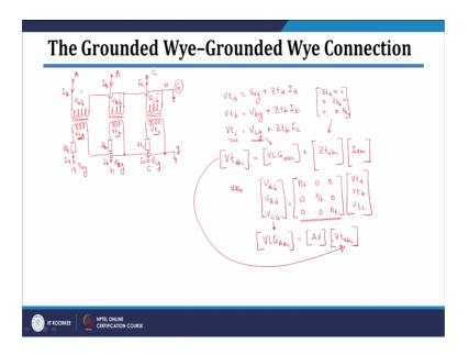
So, this connection will be something like this joining say these are the three transformers here ok, then as I told you we are linking this impedance on the secondary side. So, impedance of all the three transformers I am just showing at secondary side and since we are going to connect them in star both the winding.
