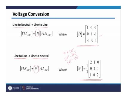
Then we have seen that many times since we are considering three-phase modeling. Many times we need to convert your line to line voltages to line to neutral voltages or delta phase current to the line current and line current to the delta phase current ok. So, we need to know this transformation matrix, so that we can easily convert them.
