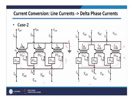
Let us say case two, where zero sequence current will be present. So, I have shown it two cases where there is possibility of presence of zero sequence current. So, in this case, we are having again this y delta transformer. However, unlike your earlier case in this case I am grounding this of y connection.
