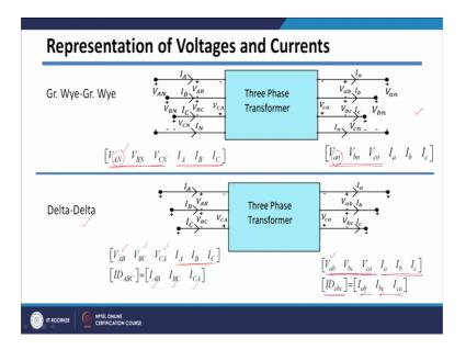
So, we have seen that the voltage which are generally represented by with respect to your ground terminal that is V AN, V BN, V CN and then current will basically your line current that is those are I A, I B and I C. And as I told you in the last class, we are using capital letters to represent primary side quantities.
