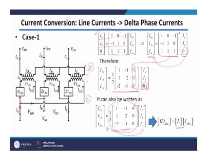
There are two cases. In case 1, if the path for zero sequence current is not available. So, in many cases only positive sequence and negative sequence currents will be present; and there will not be path available for zero sequence current. Like one combination which I have shown it here; in this particular transformer, this connection is actually star connection or Y connection and this is your delta connection. So, this is Y connection in
