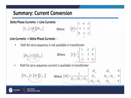
Similarly, we have got for current conversions. And two types of current conversions will required that is we need to convert delta phase current to the line currents or line currents to the delta phase current. So, two types of conversions are required. Converting delta phase current to the line current is easy; and for that we have seen that we can use this K matrix we have derived also
