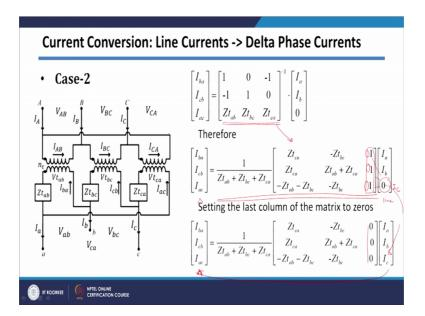
So, to get delta phase currents, I need to take the inverse of this matrix. And inverse of this matrix can be calculated which comes this one. So, this is basically this inverse here. In this case also, we are now getting required currents; here we are getting delta currents and here we are getting line currents. However, this one term I C is missing.
