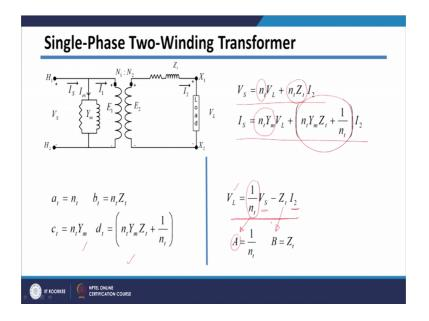
In the last class, we have seen two equations which we have written by seeing your equivalent circuit. And from these two equations we get a, b, c, d parameter. So, what we have got a, b, c, d parameter. This is a parameter; this is your b parameter; this is your c parameter; and this is your d parameter. So, I have written them here
