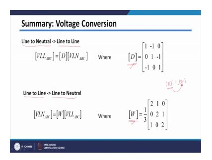
So, this gives me line current to the delta phase current conversion. So, in summary of this lecture or last two lectures, we have seen various conversion matrices which are required, because as I told you or most of the transformer which are in distribution system mostly they will be three-phase transformer and they will be unbalanced and you need to model actual three-phase transformer. So, whenever modeling actual three-phase transformer, we need all these conversions.
