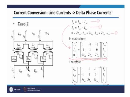
So, let us say this is equation number 1, which I have got; the equation number 2 and then equation number 3 which we have got on last slide I am taking it here. We can put them into matrix form. So, if you put these three equations into matrix form I will get this term here, so this matrix (Refer Time: 21:29) equation.
