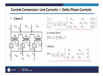
And I am calling this matrix which we have got here I am calling matrix M. And this matrix M is actually basically represented by this one.
