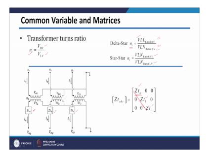
Let us see some terms, which are related to different derivations for different configurations. Before going to this configuration, let define some terms so here I defining turns ratio so turns ratio is defined. We are defining or we are using the terminology that voltage rated voltage on HV side divided by rated voltage on LV side, I am calling as a turns ratio.
