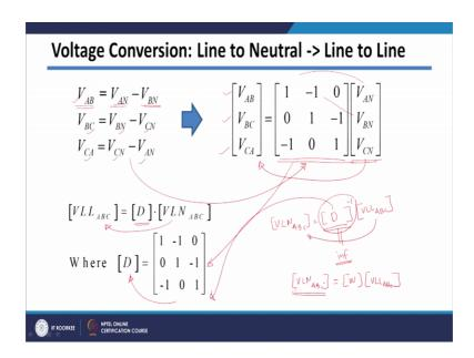
Since, it is we are considering totally unbalanced kind of system, which is having all the types of current for positive sequence 0 sequence negative sequence. So, let us see first conversion that is line to neutral to line to line voltages. So, if you want to convert line to neutral to line to line voltages so we know that line to line voltages V AB. We can write as V AN minus V BN. Similarly, V BC V BN minus V CN, V CA will be V CN minus V AN.
