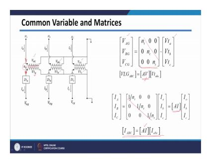
Then, the winding voltage ratio so, basically the voltages or cross the windings or always related by your turns ratio. So, the voltage V AG here and Vt a they will be always related by your turns ratio.
