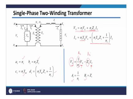
So, once you get into required form. So, this will become your a parameter, that is n t here, this will come your b parameter n t into Z t, n t into Y m will be your c parameter and these bracketed term n t Y m Z t plus 1 by n t is your d parameter.
