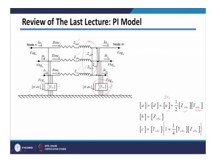
However here since there are all three-phases as well as their shunt admittances of all the three-phases are existing each of these entries they become 3 by 3 matrix; So, here this unity matrix which is actually 3 by 3 unity matrix. Z abc is matrix of 3 by 3, which consists of your all the line impedances and the mutual impedances between the line.
