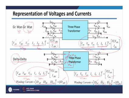
So, Wye-Wye connection which is having both side ground connection. Now, this I am representing it or you can say this neutral is grounded here. Then primary voltages basically phased to ground voltages or phased to neutral voltages they are V AN, V BN and V CN which are represented heat here and then there are line currents I A, I B and I C I written it here.
