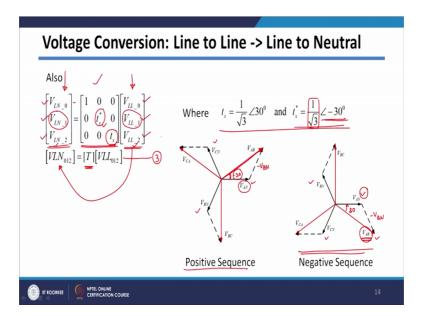
And third equation, we can get it from relation between line to line sequence component and line to neutral sequence voltages. So, this is nothing but line to line sequence voltages and line to neutral sequence voltages. So, this is line to neutral 0 sequence voltage, line to neutral positive sequence voltage, line to neutral negative sequence voltage.
