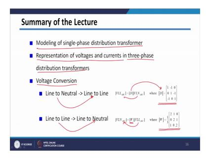
So, in summary of today's lecture, we have seen modeling of single-phase distribution transformer, then we have seen how we represent voltages and currents during modeling of three-phase distribution transformers. And for that, we need various convergence, two
