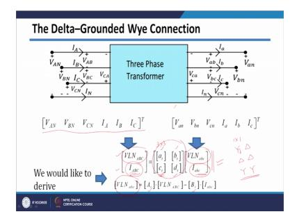
So, this is actually represented, representation of various voltages and currents in star connections and delta connections. The winding is a delta and grounded Wye. So, some transformer says primary side is delta and secondary side is grounded Wye. Then your terms will be, these terms will be on primary side and these terms will be on the secondary side so this is actually representation.
