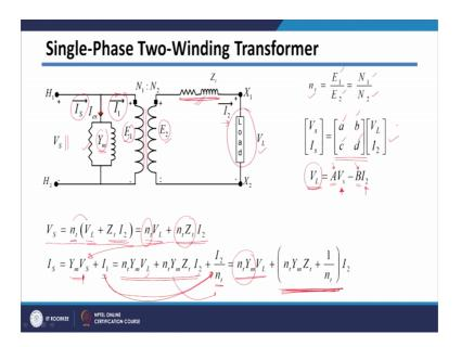
So, to put that let us see this transformer single-phase transformer two-winding transformer. We know that there is magnetizing branch since it is shunt branch; I have shown it using admittance Y m. Then, there is ideal transformer, which is having the internal voltages E 1 and E 2, load voltage V 1 V 1 and then load current I 2.
