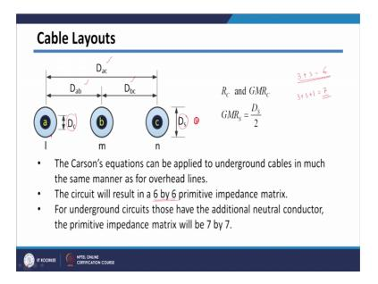
Let us say diameter of your conductor is Dc and diameter of your shield is Ds of for each of the cable. Now if you observe here there are 3 conductors those are abc phase conductors and as I told you your shield is grounded.
