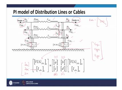
So, here I have shown the 3 phase conductor, because as I told you we need to model since the lines are not transpose as well as there is always unbalance in a distribution system we need to model a distribution system 3 in 3 phase mode. So you need to model each phase; so, these are 3 phase conductor after applying the Kron's reduction and after eliminating your ground conductors.
