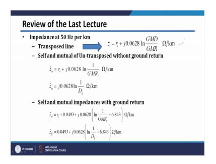
However, in case of un transpose line basically we have seen that in case of distribution system lines are untransposed; because they are short length lines. And if you are considering un transpose line and if their balance means if there is no ground return
