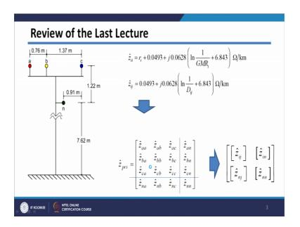
And then using these equations we have seen that how to calculate your primitive impedance matrix by knowing the GMRs; GMRs of various conductors and distance between the various conductors and using this Carson's equation, we have seen that we can get primitive impedance matrix. And this primitive impedance matrix as I told you it will be number of conductor by number of conductor size and if you apply this for the figure which is in the right hand side.
