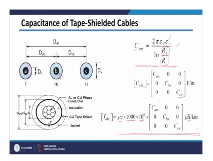
So, this is how we calculate impedance of the cable let us see how we can calculate capacitance of the cable. Now capacitance of the cable will be easier because if you see the electric field distribution due to application of voltage to the conductor, it will be just between your conductor and shield. So, electric field actually will not go out of the cable.
