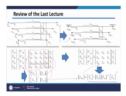
And Kron reduction we have derived one equation which gives.so, first we have seen we have to separate out terms which are related to phase quantities or phase conductors.
