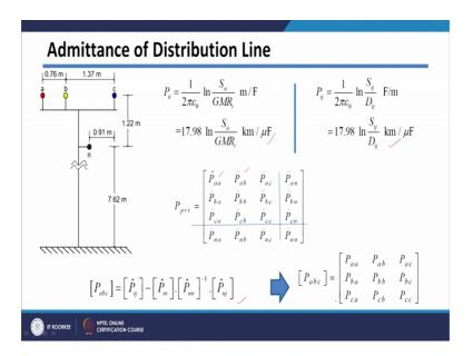
So, let us say again for that example, which you have considered for impedance calculation how can we calculate the potential coefficient matrix.
