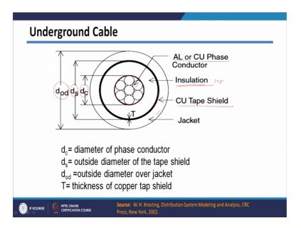
On that standard conductor to equalize the feeders to smoothen the field, we know that there is conductor shield they place it on it, and then there is insulation and after the installation again there will be cooperative shield.
