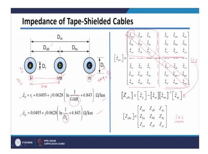
As I told you whatever Carson's equations which you have derived, you can use it for calculation of each entry of your primitive impedance matrix. So, each of the entry in primitive impedance matrix can be calculated by using this one. So, to get the diagonal entries of this primitive impedance matrix basically these entries, we can use this equation and in that case you need to use GMR of the particular conductor.
