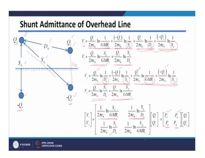
So, here I have consider say 2 conductors say conductor i and this conductor j, and we know that for calculation of the capacitor we need to take ground effect into account and for that we have seen that, we need to use a method of images. So, what we do in method of images, we take the image of the conductor with negative charge. So, image of conductor having charge Qi we have taken this image which is having charge minus Qi.
