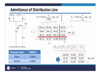
Let us see how we get it. So, by using this equation I can get these potential coefficients, I have calculated for these cases and as you are seen that the unit of these potential coefficient matrix is kilometer per micro farad and then we can use Kron's reduction.
