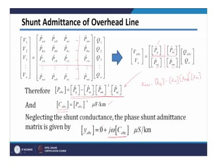
So, in this case also we can divide this matrix by knowing the ground conductor and phase conductor we can separate this matrix into 4 parts. So, these are the 4 parts of matrix and here we know that this P ij's are the coefficient which are related to phase conductors and in this case these all these matrices which basically belongs to the mutual potential coefficient and self potential coefficients of between your phase conductor and neutral conductors.
