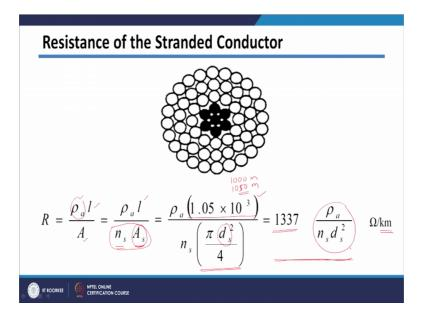
However, we have seen that our actual conductor is not a single conductor earlier formula was applicable for only the single conductor.
