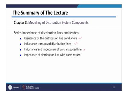
So, in summary we have started the chapter number 3 which is modeling of distribution system components. And we have started with first component that is distribution feeders and distribution lines and we have started with calculation of impedance of this distribution lines or feeders.
