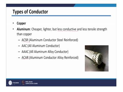
And nowadays since aluminum is cheaper and lighter it is widely used; however aluminum as I shown it here aluminum is less conductive and it is having a less tensile strength. Means long conductor will be requiring a higher tensile strength because we are
