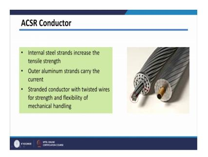
So, steel strand will be at the middle which are basically give to increase the tensile strength. And the aluminum conductor, which are at the outer part they are basically to carry the load current ok. So, as you know resistance is calculated by using this formula.
