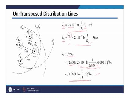
Let us see how to calculate mutual inductance. So, for mutual inductance I am considering here flip linkages due to current ij; so, flip linkages of conductor I due to current in conductor j. So, any conductor j the current is ij here and flip linkages of conductor i due to current j is given by this formula which is 2 into 10 raised to minus 7 natural log of 1 divided by D ij; D ij is nothing, but distance between conductor i and j.
