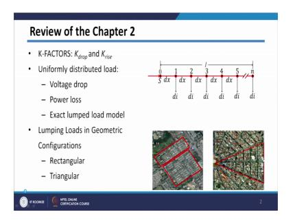
Those are K drop factor and K rise factor and we have seen that K K drop factor is nothing, but a percent voltage drop per kVA per kilometer and it is basically used to find
