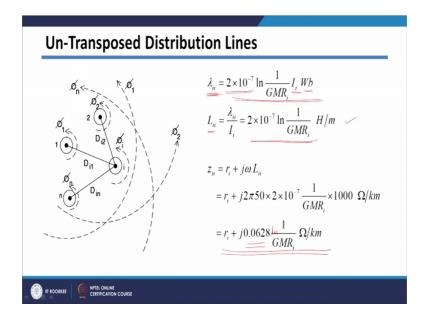
However, we have seen that our distribution lines are generally un transposed because they are short length line and transposition only done the length of the length is length of the line is longer. So, in case of distribution feeders they are generally un transposed; so, if there are un transpose feeders and if there are n conductors in the system, then there will be n by n matrix because there will be a self inductance mutual inductances we have to take them separately.
