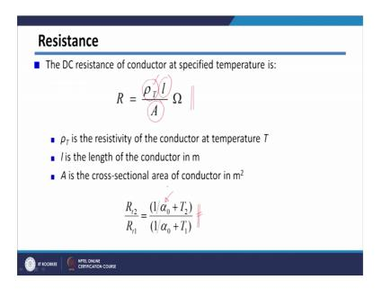
Where this rho T is actually resistivity of the conductor material this is length of the conductor and area of cross section of the conductor. And as you know that resistivity of the material is temperature dependent, so resistance will also change whenever temperature is changing.
