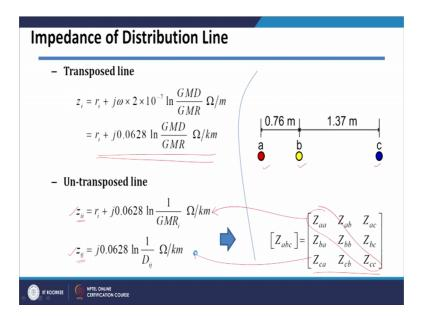
So, in summary we have seen that in case of transpose line we have only one impedance value which is given by this situation here. And in case of un transpose line as I told you will be having n by n matrix if there are n number of conductors into the system and this n entries of n by n matrix will be given by this formula, where this z ii will give you a self impedances of those conductor and z ij will give you mutual impedances between the conductors.
