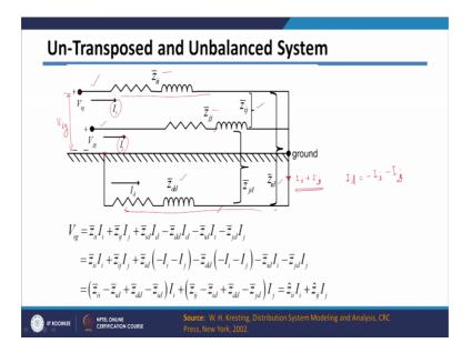
This is a one conductor I another conductor is say j Z ii is self impedance of conductor I Z jj is self impedance of conductor j and Z ij is mutual impedance between them. Now I am considering the ground also as a one conductor because it is carrying your unbalance neutral current in that case earth will act as a another conductors.
