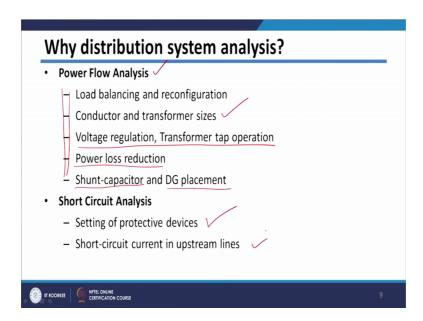
Now, we will see where the distribution system is required or where it is applicable or where it is used. So, as I told you the basic analysis is load flow analysis and short circuit analysis. So, load flow analysis is required for taking various decisions during operational stage of the distribution system as well has design stage of the distribution system.
