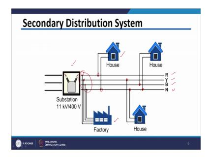
Similarly, there is one commercial consumer which is shown it here which is 3 phase; if you see the secondary distribution system secondary distribution system start with 11 kV by 400 volt substation and it is basically 3 phase 4 wire system. So, there is there are 3 phases R Y B and one neutral phase. So, 3 phase 4 wire system it will be providing power to the some big consumers as well as some domestic consumers like our houses.
