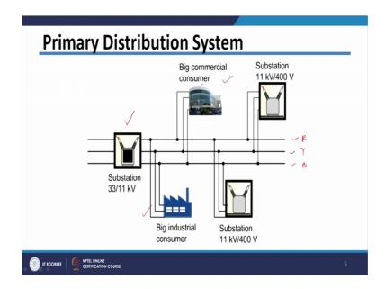
Now, if you see the structure of your primary and secondary distribution system which was seen earlier. The primary say distribution system basically consist of your 11 kV network, we also call it has HT level; High Tension lines. It starts from your 33 to 11 kV substation and it will be basically 3 phase 3 wire system.
