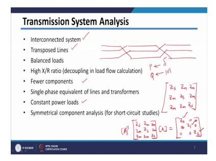
Now, we will see transmission system analysis. So, basically in this particular slide we want to see what are the assumptions we are made, during the transmission system analysis. So, we know that the transmission system is basically interconnected kind of system. So, your algorithm should be such that this interconnection or loop kind of structure it will take into account.
