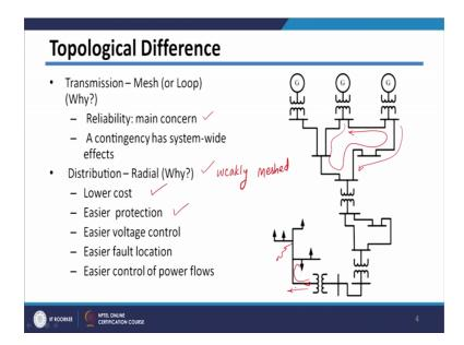
Your distribution system will be radial one radial means it will not be forming any kind of loop or it is kind of weakly mesh system. Weakly meshed means there will be only few loops unlike in case of transmission system. So, since transmission system is highly inter connected kind of system.
