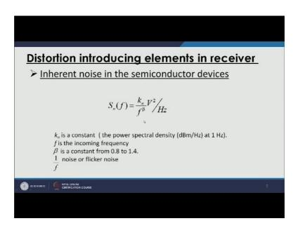
So, this is the formula for this noise. So, this noise if it is shown, as a function of frequency then, it is proportional to a constant k n, which is mostly power spectral density taken at hertz of the frequency. It is proportional to the square of the input incoming voltage applied and, it is inversely proportional to the frequency it to the power beta. Now this beta is a constant, which is taken from 0.8 to 1.4 and 1 upon f is a specifically called flicker noise or 1 upon f noise.
