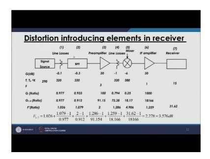
As we can see here, that we have at this signal source and our first input noise is coming from here, then the noise losses, they are making the first stage, there is a band pass filter it is second stage, free amplifier third stage again, there is a line at has losses then it is fourth stage, mixer has the fifth stage, IF amplifier at the sixth stage and then, eventually the receiver in the additional domain it is seventh one, seventh portion.
