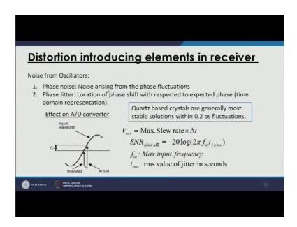
So, phase noise is something, which is a kind of noise, it is the rising from the fluctuations and, if these situations are seen in the time domain and we can compare it with the original point of the phase, then it is called the phase editor.
