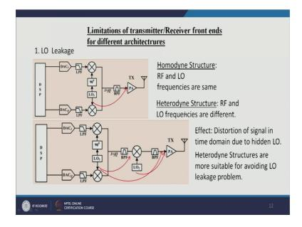
In heterodyne structure we can choose our RF frequency is separate from the RF frequency. So, what is LO leakage, basically when we are putting our signal in the contacts your phase by using a LO, then some of the LO might directly leak into the direct path.
