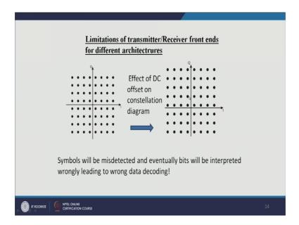
In the LO we can see the destruction was there, because of the DC offset in the constellation diagram we can see that the constellation shifts in one direction, and shifts in the direction where actually our amplitude is being added.
