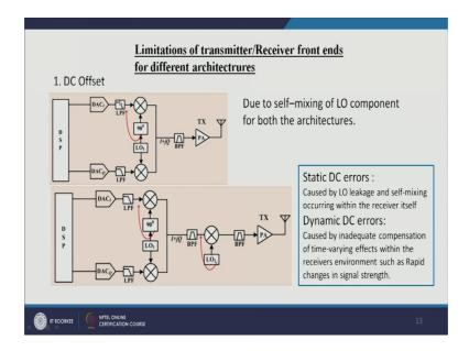
Now look at the DC Offset. Actually DC Offset is again after effect of having the LO leakage. Now LO is leaking from this part to the previous to the mixing path.
