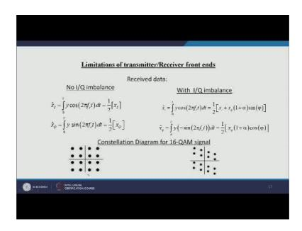
Whenever we get our signal output signal we multiplying the cosine factor and take its integration over 0 to t and do the low pass filtering.
