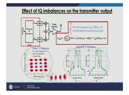
We have just given the fc which is the carrier frequency. So, we are not giving it a ie frequency there. In this case, our image is hiding inside it and we are showing our component alpha which is showing the gain imbalance and this phi which is representing the phase imbalance in the system. This Ci Cq are actually dc offset which we have discussed earlier.
