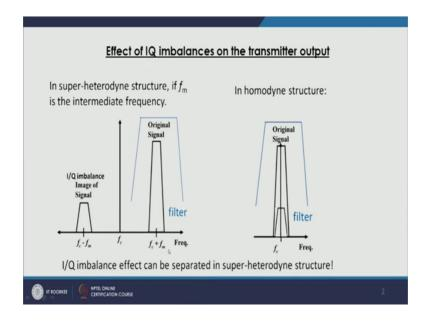
Original signal at fc plus fm which where fm is denoting your intermediate frequency because, of the IQ imbalance you will see one component and image of the signal at fc minus fm. Higher the IQ imbalance and higher will be the magnitude of this IQ imbalance image signal.
