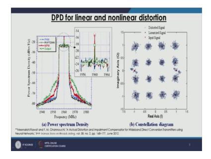
We are able to get the auto of band distortion in control and there are some results, in the right hand side, we can see the constellation diagram and the red marker here, circle is was the original input the distorted signal because of the IQ imbalance in the PA nonlinearity is the blue one and after linearization by using our model and digital model this black signal is falling clearly on top of the original signals. So, it has got perfectly in the real practical scenario.
