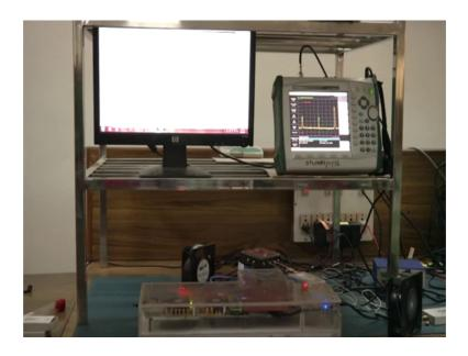
So, this is the setup which is using an FPGA and this FPGA can interacts with transmitter as well as receiver both of them. We are using 2 fans here and we are using power supply to provide the supply like 6-volt, 5 volt, etcetera. Whenever it is required apart from other receiver we are using an extract spectrum analyzer as a receiver. So, that we can observe the performance at the output of the transmitter and we are using personal computer for doing the processing of the setup.
