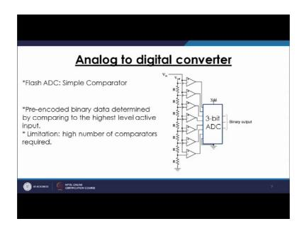
This is a simple example of the analog to digital converter. Again, they are much more sophisticated examples than this, but it how the working of the ADC is done. Basically, it is a simple competitor what is happening in the circuit again it is 3-bit ADC. The example we had done earlier for the 3-bit DAC it is opposite to that 1. Our data is in the form of voltage and you want to get about binary digit out of it.
