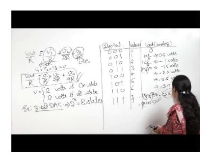
Right. If I choose my V1 is equal to V2 is equal to V3 equal to a fixed voltage then basically V out can be given as V out upon R is equal to V upon R plus V upon 2R plus V upon 4R.
