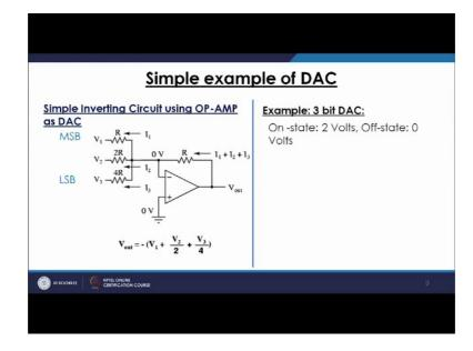
This example shows a simple inverting circuit using OP-AMP as digital to analog converter. What is the fundamental of this operation? If we look here this operational amplifier it has a V out and it is attached as a inverting mode. Now that inverting voltage is given as 0 volt. With respect to this 0 volt, there are 3 branches each branch contains a different resistance.
