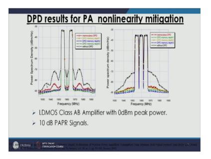
In this case when there is no DPD, no distortion was there this black curve is showing power amplifier output and we can see that auto of band distortion is here it was the original signal. 3 carrier signal which has one missing carrier and third carrier, if 3 carriers are on for this wedma signal we can see this is the profile and this is the auto of band distortion which can which is comparing because of the power amplifier.
