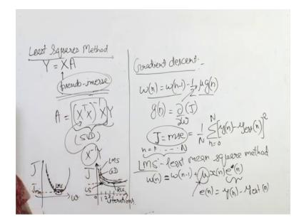
So, by using pseudo inverse of this X you are able to get dual coefficients. So, it is one step process because once you have defined your Y and X observation matrix in one step for n data you will have single solution.
