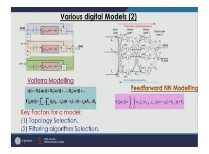
So, they are several filtering algorithm in the literature, but first of all we have to see how we can apply those algorithm. For example in linear filter theory we have some of the examples where we do the fitting and in our Wiener Hammerstein's model we are using a fir. So, we will start our discussion from the fir filter there fitting and then we will take the non-linear to linear mapping for the memory polymer model and we will show how we can apply those in the non-linear terms.
