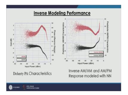
So, here for a practical system Doherty power amplifier we are showing the actual PA characteristic, so in the left hand side figure we can see that our AM, AM is given by this red curve which is the gain, and just normalize gain, so this around 0. We have removed the small signal gain so that we can just see its performance.
