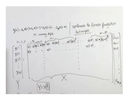
No, observation matrix will contain x 1, x 1 at absolute of x 1 and so on for n equal to 0 right.
