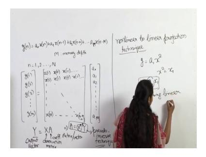
So, for a fir model our y n was a function of input signal and its previous values of the input signal m is memory depth here. So, basically we can represent the same thing as a matrix also. So, if we take different value of n from n, n equal to 0 to 1, not 0, it will have integral value positive integral value 1, 2 up to n.
