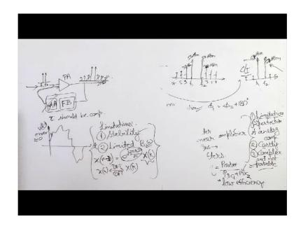
So, in this technique basically, this is your power amplifier and we say, that distortion is occurring at the output power amplifier output. So, suppose these are the input signals. So, at f1 f 2 and these are the imd components at the output
