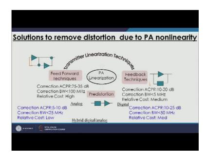
We are showing different transmitted linearization techniques the basically, there 3 types of techniques which are found in literature. One is called feed forward technique. Another is called feedback technique. And a third one is called pre-distortion technique.
