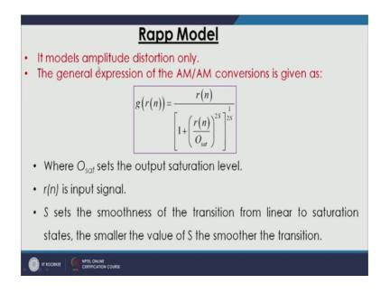
Basically, it focuses only on the gain distortion. So, it does not cover the phase distortion. So, general expression for the AM AM conversion is given as g r n, which is the gain, with respect to input signal amplitude and if you see here, it has input signal amplitude here and apart from that, it has Osat which is the output saturation level.
