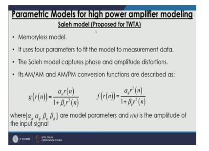
Proposed for TWTA it is a memoryless model, means output is a function of input itself and not the function of it is previous samples, it uses 4 parameters to fit the model to measurement data, it captures phase and amplitude distortion separately and independently and this functions are defined by g r n and f r n. So, this g r n is AM AM or the gain in the voltage form, when I say gain the voltage from it, means it is not a dB.
