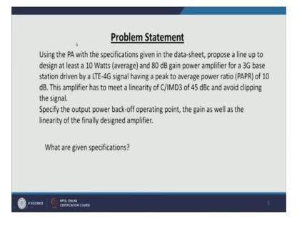
We have to use the PA with the given specifications in the datasheet, and we have to propose the lineup to design at least a 10 watt average power and 80 dB gain power amplifier for a 3G base station, which is driven by a LTE 3G or 4G signal, main requirement here is that the signal has a peak to average power ratio of 10 dB, this amplifier has to meet a linearity of C by IMD 3 of 45 dBc and it has to avoid clipping the signal.
