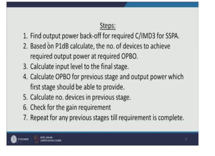
First of all, we have to calculate the output power back off, for required C by IMD 3 for solid state power amplifier, now looking at our problem statement we require at least 10-watt power from our power amplifier. So, let us converted back into dB logarithmic scale, because most of the calculation will be in terms of dB and if you see C by IMD provided in terms of dBc and our gain of the power amplifier it is given in terms of db. So, let us calculate this output power into dB first of all.
