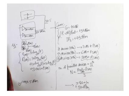
Now, this particular PA which we are studying and specifications are given here, we are able to get only 24.5 dBm from it is output, because we have to maintain the C by IMD 3 ratio of 45 dBc, but we have to achieve 50 dBm from the system. So, how can we do that.
