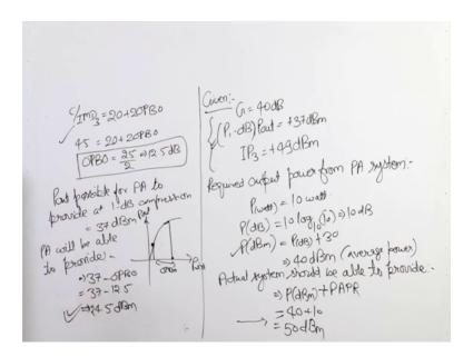
So, required output power from PA system, I am calling it system because eventually we will select number of power amplifiers to make this system. So, the P in watt is given as 10 watt. So, P in dB will be 10 log 10 10 is actually 10 dB and P in dB m, will be P in dB plus 30 this was a relation. So, 40 dBm so we should be able to get 40 dBm average power, now it is also given that we should avoid clipping of the input signal and the signal has the peak to average power ratio of 10 db.
