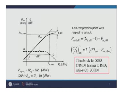
If we see here the relation between IP3 and P1 dB for the SSPA, it is given by this formulation means P1 dB is equal to actually IP3 minus ten. So, if we knowing the IP3, we can calculate our P1 dB from here, but in this case, we know both of them we know our IP3 and we know our P1 db.
