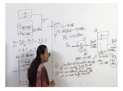
The gain of the stage and the linearity of the finally, designed amplifier. So, G is 40 or both of them OPBO was 17.5 dB here and the previous stage here it was 50 minus 12.5. So, it was I think 15.5 dB we are maintaining C by IMD 3 of 45 dBc, because we have done our calculation for keeping this linearity requirement, and we are getting our output requirement of 50 dB m. So, our signal is not being clipped and we are able to design the system completely.
