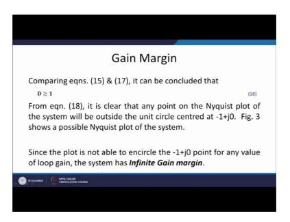
So, since the plot is not able to encircle the minus 1 j 0 point for any value of the loop gain, the system has the Infinity Gain margin, but they are may be the other condition that is a unit circle. So, my this point will be minus 2, 0. So, on the higher side; my gain
