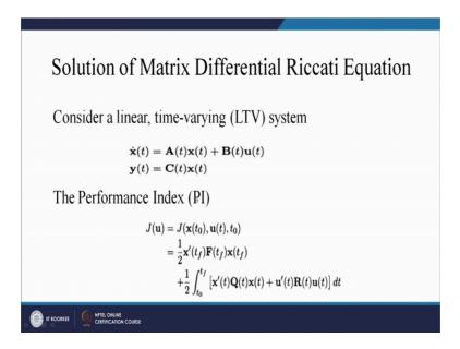
Our approach was for a given system x dot equal to x plus PI equal to C x. We are finding out the u t by minimizing the performance index as half of x prime t f f of t f x of t f plus half of integral t 0 to t f x prime t Q t x t plus u prime t R t u t. So, we have to minimize this performance index subjected to the plant. Objective is to find out the minimum value of the u.
