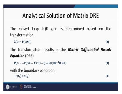
So, a transformation matrix is lambda t P t X t and my matrix differential equation I am writing as P t A minus A prime P Q P B R inverse B prime P with boundary condition is P t f equal to F of t f.
