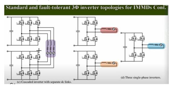
Here also six links are there and in this case also six links are there. But here what is the difference? The DC link are separated. So, it is divided in two DC link rather than one DC link. So, here it is DC link and DC link Okay, so now it is like conventional voltage source inverter.
