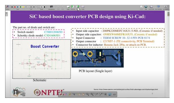
Now, In this particular lecture, I am going to discuss the same boost converter which was used for simulation in LTSpice software. If you don't remember, you can go back to the lecture and you can just see the boost converter. So, say the boost converter here, it is given the schematic of the boost converter. So it is having switch and the diode model they are same as it is used in LTSpice
