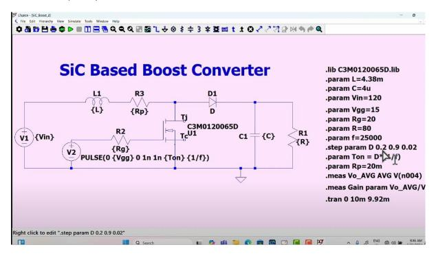
In order to find out gain, so here one parameter is even defined here, the gain parameter. So, what is this gain parameter? So, gain parameter it is V0 average because you know it is having V0 is having some ripple. So, that is why we need to use V0 average to get the
