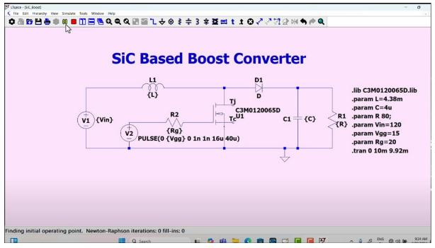
So, now, then we have to run the simulation. Running the simulation, you can see here, this is the part which I already told you, you can run this simulation.
