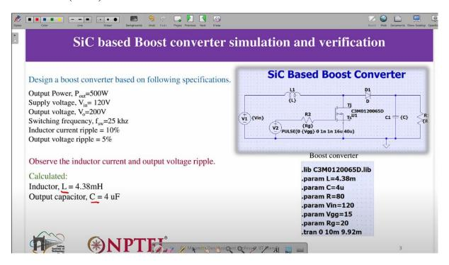
So you can see here so this is the simulation we have considered so efficiency in this case is considered as 95 percent, right? So, this much you can actually calculate. So, we can just check this input voltage and current in the simulation, output voltage and current and that much efficiency is visible or not that you can consider.
