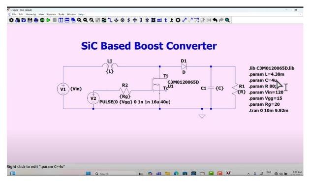
But if you write m then it will consider as milli henry and similarly for capacitor you can see this is kept as 4 micro that means it is 4 micro-farad. So, same way you can actually define the parameter as it is suitable for you. So, in this case the resistance which is considered as the load resistance it is kept as 80 and the input it is given as 120. So, that is the thing is kept here. And then here the important thing is that Vgg, it is the gate voltage. So, this gate voltage you can
