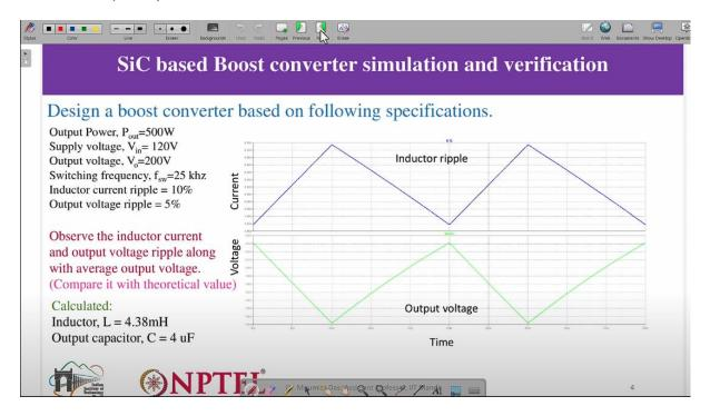
So, this is the part which I have showed you in the simulation itself. So, inductor ripple current at the output voltage, output voltage ripple and the inductor current ripple this is something which we have actually considered.
