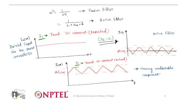
so generally what happens whenever we try to use the passive filter so then what happens omega we represent as the like the frequency, cutoff frequency. So, what we do? So, omega we try to find out it is equals to 1 by root under LC or omega square equals to 1 by LC, right.
