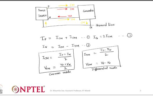
So, now if I try to analyze these noises, so then how I can analyze? So, I can just draw the block diagram again.
