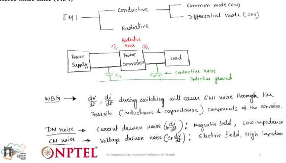
so the EMI, so EMI we have seen we can actually classify in two types, right. So, conduction mode EMI or conducting type EMI and then radiative EMI. Now in this also there are two different types of EMIs in conductive type.
