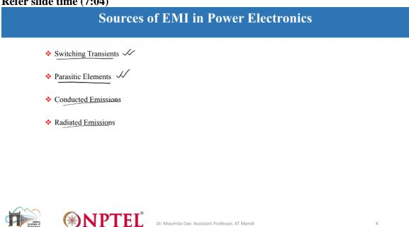
So, basically if you consider any power electronic system, the main component is switch which is the which is basically heart of the power electronics system. So, then these switches will cause switching transients to be present and this switching transient is one of the main of the **EMI** noise. reasons
