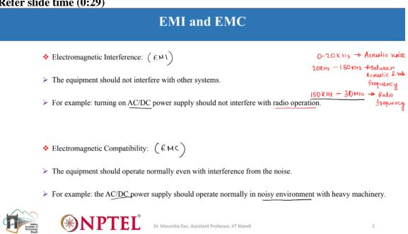
Say about electromagnetic interference or electromagnetic compatibility, we first have to know how these problems are coming. So as you can see in this particular slide, it is written electromagnetic interference which also known as EMI. So it is basically the equipment should not interfere with other system. Suppose we have any equipment.
