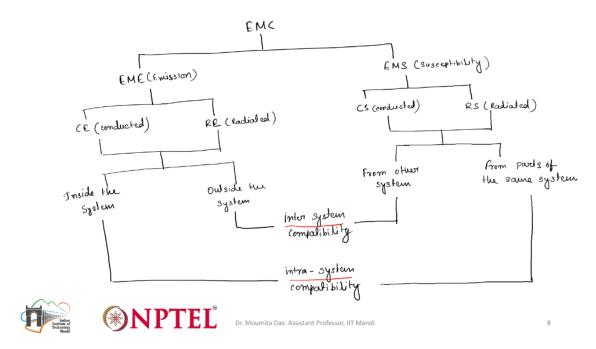
This is with respect to susceptibility. So I am just writing the short form. And this is with respect to the emission, electromagnetic emission. Now this electromagnetic susceptibility again can be classified into two types. So that is conducted susceptibility.
