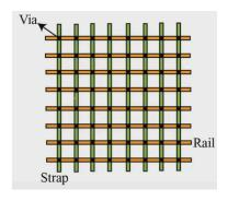
Now these networks or this mesh basically carries the VDD. So this may be for VDD there will be another mesh for say ground line, and from this power delivery network or mesh grid the power pins of the standard cells and macros will be driven and those will be tapped from these lines . So this is how the power delivery network is created over the entire core area and from the core from this power delivery networks the from appropriate tapping points we get the we we get metal lines and then that
