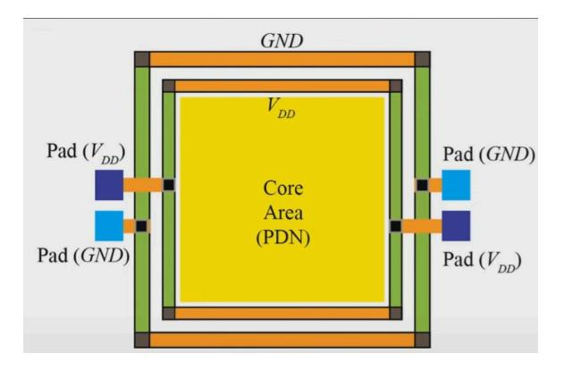
Now these are the power pads. In this case I am showing there are 4 power pads. These light blue ones are ground power pads and the dark blue ones are the VDD power pads. Now from these power pads we have 2 rings, one ring for ground and another ring for VDD, . So, the power rings carry power around the periphery of the die. Now for these ground lines or ground rings and power rings which layers of metal do we use? Typically we use the top layer, top most layer, .
