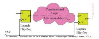
The one which is launching the data that is known as the launch flip-flop, and the one which is capturing the data is known as the capture flip-flop. So this is the capture flip-flop, and this is the launch flip-flop. In a synchronous circuit, the data that is launched at a particular clock cycle that should reach the D pin of the sequentially adjacent flip flop by the next clock cycle or next clock edge.
