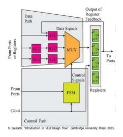
It has two distinct parts: the data path and the control path. In the data path, major portion of the computation is done. For example, there are ALUs or arithmetic logic units which is doing a kind of computation. These units can be adders, multipliers, or logical units like AND gate, OR gates. These kinds of logical operations will be performed in the data path.
