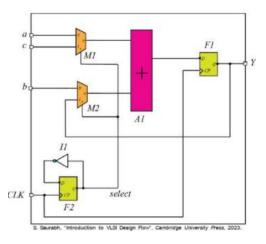
Now, the adder is being used to compute a + b in one clock cycle. Whenever select is equal to 0, then a and b come to the adder input, and you get the result as Y = a + b. Whenever the clock comes, the output is a + b, and this is fed to M2. And whenever the next clock edge comes, what happens is that since Q is connected to D through an inverter, this Q will toggle every clock cycle. So in one clock cycle, it will be 0, then in the next clock cycle, it will be 1, then 0 and 1, and so on.
