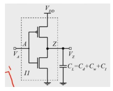
So if it is a CMOS inverter, this CMOS inverter will internally consist of a p MOSFET which is shown here and an n MOSFET right.
