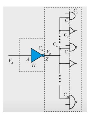
as C d right. So, these are the various components of the capacitances which will be charged and discharged as the input of the inverter is changing.
