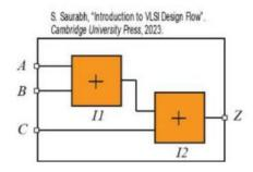
For example, consider this circuit. In this, there are two adders. The first one is adding A + B. The result is produced here as A + B, and the second adder is adding (A + B) +C, and the result A + B + C is produced by the circuit. But this second adder can do the computation only when the first adder has done the computation.
