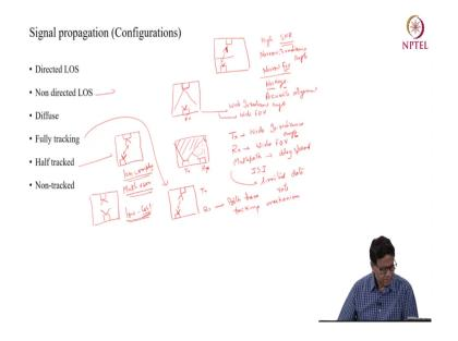
So, before going further let us discuss what are the different configurations of light propagation inside a room for example. So, it could be a directed line of sight. So, when I what I mean by directed line of sight? So, you have for example, this is your room and say this is your transmitter and your receiver is for example say here.
