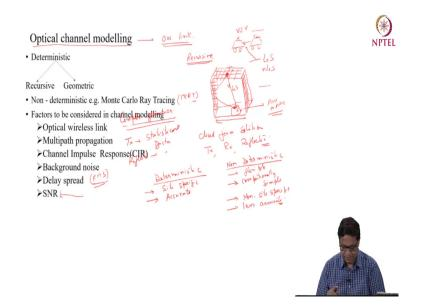
So, now let us understand the optical channel modelling. We need to calculate this accurately so that you are able to understand about the optical wireless link, the performance of optical wireless link. And optical for optical channel modelling there are two methods one is deterministic approach, under deterministic we have 2 types recursive and geometric and the other approach is non deterministic Monte Carlo ray tracing.
