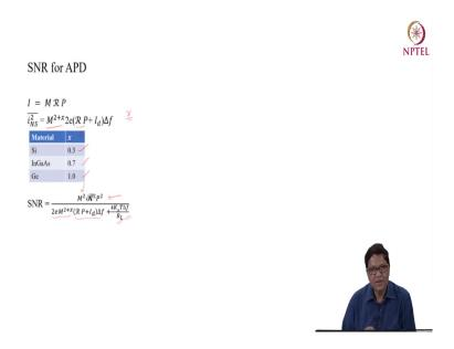
Now, let us calculate the signal to noise ratio for APD, as we discussed last time that APD gives you a gain of M there is an amplification gain because of the avalanche effect. So, the current which is produced is M times than what it is produced in a PIN diode. So, it will be M responsivity into power and the shot noise current will be again there will be increase of shot noise current, because the there is a avalanche effect.
