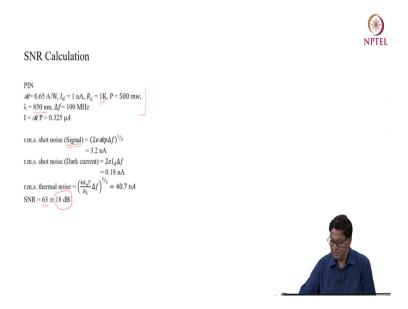
So, now let us now try to calculate the SNR for a PIN, PIN diode first and then we will calculate SNR for APD. So, for PIN again assuming some typical values of responsivity id dark current assuming load resistance as 1 kilo ohm and 500 mill watts of power and suppose I am working at 850 nanometer and the bandwidth is 100 megahertz.
