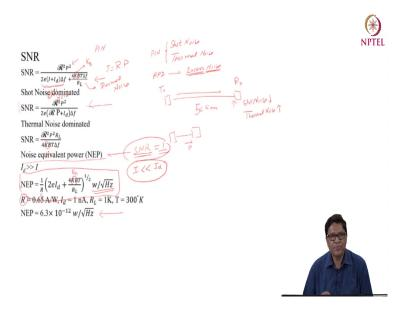
So, the NEP expression is given in this fashion and if I want to calculate the value of NEP for typical photo diode where I assume responsivity as 0.65 amperes per watt, dark current is 1 nano ampere and RL 1 kilo ohms and temperature of 300 degree kelvin; I get NEP as 6.3 into 10 raise to power the minus 12 watts or 6.3 pica watts per square hertz. So, this is the value of ne NEP.
