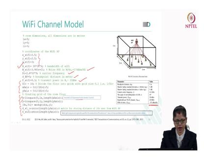
So, let us see the simulation here. So, whenever we have simulated this a WiFi channel we have considered the same like room size of 5 like length of the room size, breadth of the room size 5 5 and the height of the room is 3 meter. Coordinate of the WiFi access point we have considered at the middle of the ceiling that is why 2.5, 2.5, 3. And, we have considered bandwidth of the WiFi access point is 20 mega hertz and power spectral density as per this reference we have considered.
