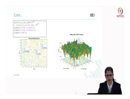
Finally, we have the SNR values of the user from the AP whatever we are getting at each grids. We can plot it by using the surfc as we have done in the case of LiFi. So, we will get this is the SNR profile for the single WiFi AP in each grid of the floor. So, we can observe here we are getting the 81.019 dB if at this location and here we are getting 9.8 that means, here the user is getting very less SNR.
