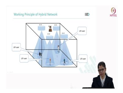
So, let us see how the hybrid network works. This is one small scenario has been taken here. We can observe here this is one room and under room ceiling, we have placed four LiFi APs and under that LiFi access point some users are available and here we can see that user 1 is static and user 4 is also static user 5 and user 2 are mobile. So, at one position then those LiFi users are under the LiFi access points therefore, they can get the signal from the LiFi access points.
