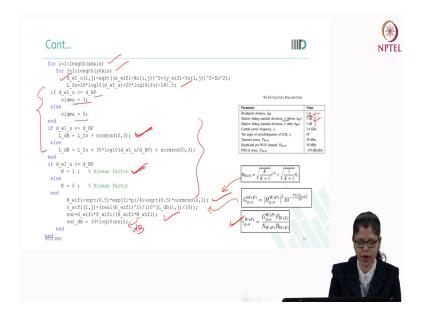
So, similarly in LiFi how we have considered we have a considered two for loops because we have to calculate the channel impulse response and channel gain at each grid that is why we have taken these two for loops. Then we have calculated this distance between WiFi AP and user by using this x minus Xu whole square plus y minus Yu whole square plus Zu square using the geometry the value we have calculated.
