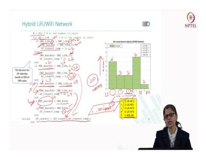
So, here we can see that the notation we have used 1 for LiFi access point, 2 for LiFi access point 2, 3 for LiFi access point 3, 4 for LiFi access point 4 and 5 for WiFi access point these are the connectivity we have considered in this. So, finally, we can see that we will be getting the result of the connectivity of each user for the five access points whatever we have used in our system. So, we can see here all the connectivity's are like here we have taken connectivity, number of users.
