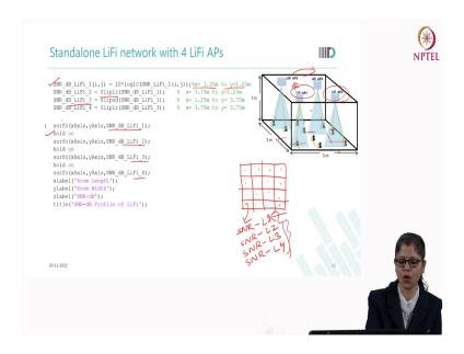
So, we can duplicate it by using the simple command like flip up flip left. So, here what we have considered? So, SNR dB we have calculated for first LiFi access point as we have calculated in the previous slide, only we have changed the location of the LiFi access point at
