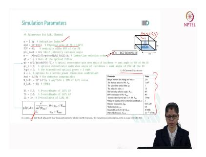
Let us see how to simulate it by using MATLAB. So, for this simulation we have used this LiFi channel model from this reference and these are the parameters we have considered for our simulation. This n is nothing but refractive index 1.5 it has taken based upon this table, APD is the physical area of photodiode. It has been taken like 1 centimetre square that is normally we can write 10 to the power minus 4.
