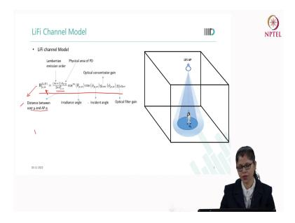
And m is Lambertian emission order as we have studied in previous lectures; APD is physical area of photodiode. This theta mu alpha is the irradiance angle for the user mu and the alpha A P a alpha ith A P and a phi mu alpha is the incident angle and g con is the optical concentrator gain and g filter is optical filter gain. So, we can see here this is the channel model which we are getting for the LiFi from the LiFi access point to the user.
