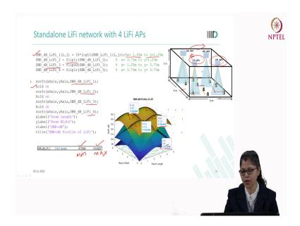
Together if we want to plot then we have to keep this hold on command and we can see the profile will be visible like this and this is the LiFi profile for all the LiFi access point and we have considered that all the grids we are receiving the data we we are receiving the SNR a value from each of the AP. So, we can see here the maximum value we are getting for the SNR is 154.4 dB and minimum value is 87.95.
