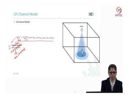
Let us see how to do the channel modelling for a LiFi network and first let us start with the single LiFi access point. Under the single LiFi access point one user is here and we have
