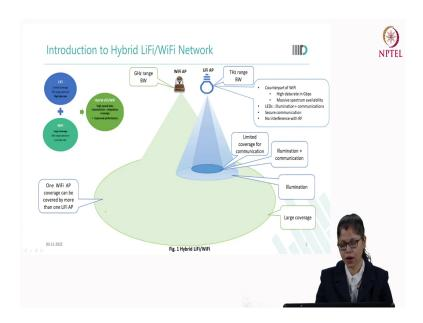
Let us start with the introduction of hybrid LiFi WiFi network little detail. So, here we can see LiFi – LiFi is a network which is having the access point repeat. Let us start introduction to hybrid LiFi WiFi network in detail. The LiFi is an access point which has the limited coverage and it operates in the terahertz range spectrum.
