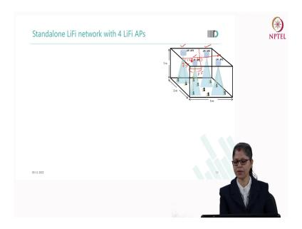
So, similarly here what we have done? We have considered single LiFi access point that is present are the like a 2.5, 2.5, 3 the coordinate the on the ceiling the access point is fixed at that point. If we are considering a room of 5 cross 5 cross 3 same and we are trying to place the first access point here, second access point here, third access point here, fourth access point here, then first what we have done?
