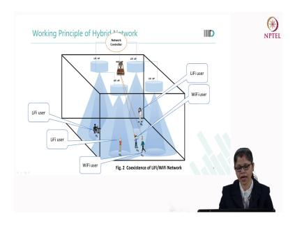
How it happens? As an example, you can see here. This user 2 is connected to this LiFi access point. And whenever he is moving, he has reached at the corner of the LiFi access point; that means, we can see that he is coming out of the at attocell of this LiFi, that time the user will get the access of this WiFi then this user can now be considered are the WiFi user.
