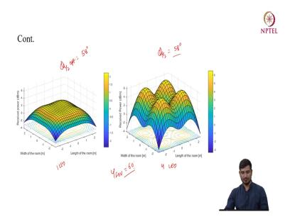
Like in our work we have tried to plot this with improved LED semi angle value or you can say the optimized Lambertian order. So, this is the 1 LED configuration with phi optimized as 58 degree and again this is with the 4 LED configuration with again phi LED optimized as 58 degree. So, this is the standard value that we have calculated you can also calculate this optimum led semi angle value as per your configuration and see the received power profile.
