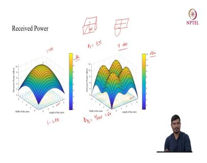
Now, now we are going to plot the 3D received power profile. So, this is with. So, this is the received power profile with one LED. It means in this case the LED is mounted on the center of the room.
