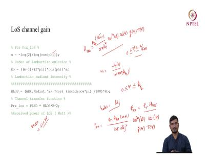
Now, we are going to simulate the line of sight channel gain. So, the first thing as you know line of sight channel gain equation is m plus 1 upon 2 pi dij square cos m phi cos psi PD gain optical PD gain concentrator gain and this psi should be in the range of 0 to field of view of the receiver.
