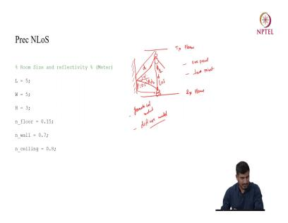
So, as you know this signal from like if this is the transmitter plane the LED is mounted here which is transmitting the power at the LED semi angle phi by 2. And suppose this is the receiver plane and there is a PD here which is receiving the signal.
