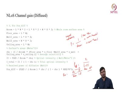
Non-line of sight channel gain as a diffuse. So, in this case we considered the non-line of sight gain with the equal reflectance from each wall. So, for that you required this. So, the
