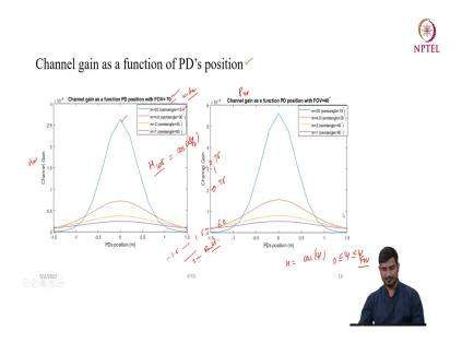
So, again you can refer to the equation your channel gain is also a function of incidence angle psi and again it is a function of cos where psi is limited between the field of view of the receiver. So, again smaller the field of view larger will be the gain, but the distances you cover will be less and the wider the channel gain you can cover more distances, but with the smaller channel gain.
