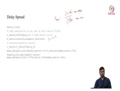
Now, as we have calculated this received power profile so, with the help of this received power profile you can also analyze the delay spread performance of the system. So, the delay spread actually the function of your received channel again only. So, as we generally know we define or characterize our delay spread with the RMS delay spread and which is nothing but t h t divided by the minus infinity to plus infinity h square t or you can say the average.
