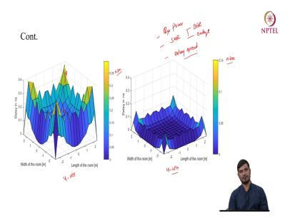
So, you can see here for different LED semi angle we have plotted this delay spread. So, the maximum value of delay spread that we are getting is 0.35 nanosecond and as we have optimizes LED semi angle we have reduces delay spread from 0.35 to 0.15 nanosecond. So, this is again for 4 LED configuration this is also for 4 LED configuration.
