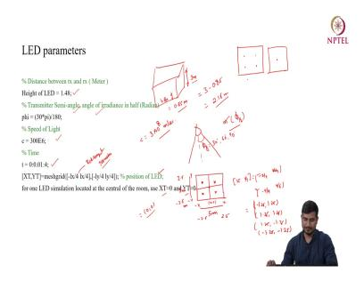
So, moving ahead now we are going to discuss one by one what are the LED parameter that we need to provide as a input. So, the first is the height of the LED or you can say the distance between the transmitter and the receiver. So, how we can calculate? So, actually generally in any practical system this height of the LED like earlier we have shown you the room size and we have given that the height of the room is 3 meter.
