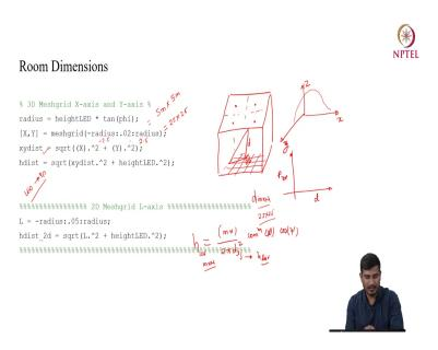
Again, like I have shown you earlier in order to calculate the received power you require this room dimension and where you are going to place the PD. So, for the same like this is the room here, what we have done is, we have already deployed the LED in a rectangular configuration and we have also identified or given input the LED parameter.
