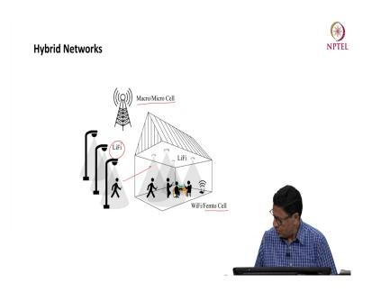
So, there are various types of hybrid networks. Suppose a user is in outside environment is connected to either a macro cell or a microcell cellular part of cellular communication. As he moves and he if he happens to be below a lamp then he may be connected with LiFi. And as soon as he enters a building you have both LiFi access point and WiFi access point or there could be a femtocell inside then this combination of LiFi and WiFi or femtocell will give enhanced performance.
