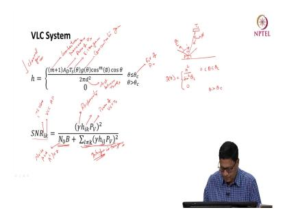
So, now let us start modeling the VLC system. So, the channel gain, this h is channel gain, this we have done many times channel gain is given by this expression where m is the
