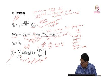
Now, let us discuss about the RF system. So, we are let us assume that RF system is millimeter wave where the frequency is 60 gigahertz and majorly line of sight. And as I mentioned the system model, we have used 4 APs, RF APs. The idea is that you know the user should be connected to a AP which has the shortest distance. So, that he gets maximum
