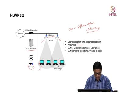
So, this is a typical diagram of a hybrid LiFi WiFi network. So, you have these are the you know for example, laptop devices and there is a dongle here, LiFi dongle and anyway WiFi is part of the laptop. So, this is the dongle the red strip you see is the dongle here and then you have these are the LiFi APs access points and also you have WiFi access points inside the room.
