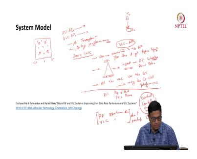
So, now let us try to understand this LiFi coexistence and let us draw the system model which we are going to study. So, system model suppose you have a room this dimension can be say minus 20 to 20 this is 0. So, about 40 meters or can be you know 10 meters or some other dimension and it has RF APs and VLC APs, VLC access points. So, VLC I am denoting by for example, this crosses these are the optical transmitters or the elimination source inside the room.
