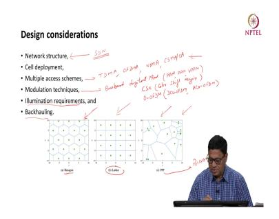
There are various design considerations while designing the LiFi WiFi architecture. The one is network architecture which I has just discussed using SDN Software Defined Networking. And then how your cells are deployed in for example, in cellular you have you know different options one is this hexagon which is very popular in cellular deployment and then you have lattice kind of deployment and then you have Poisson point process which is some random deployment of a base stations Poisson point.
