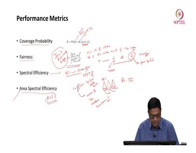
The performance metrics which are used in such networks in such hybrid networks is coverage probability. This basically is defined as probability this S stands for say SNR, a probability that S the signal to noise ratio is greater than some threshold and this alpha beta gamma are the angles of the device because it also depends on the orientation of the device.
