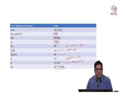
And the VLC parameters which have been used in the system is area we have taken 10 into 10 meter square and the P VLC per VLC power is 9 watts the bandwidth of the source is 40 megahertz the area of the detector is 1 centimeter square. The irradiance angle, irradiance angle is 60 degree this is the transmission or emergence angle from the transmitter irradiance angle.
