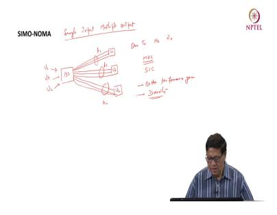
So, you can have not only MIMO, but you can have different versions of MIMO. So, one of them is single input, multiple output. So, in this what happens suppose this is the base station and these are the users U1, UL, U-capital L they are connected to base these base station. So, this information is superimposed here and then in the receiver end you have U1.
