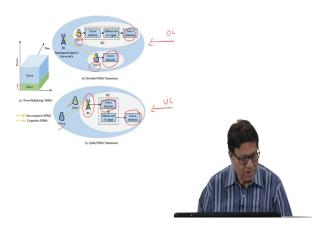
So, just to revisit uplink and downlink NOMA, so this is a case of downlink NOMA transmission; so, in this case there are 2 users. For example, user N and user M and they have different power levels, user 1 has this much power level, user M has higher power level. So, you do the SIC that is SIC operation, Successive Interference Cancellation at user N.
