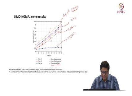
So, this is a case of single input, multiple output, NOMA. So, these are the some of the results of NOMA, single input, multiple output, NOMA. So, if you see this is user 1, this is a rate for user 1, rate for user 1 and this is user 2. This is rate of the user 2 and the sum rate is given by this curve, this is a sum rate. And if you see the conventional orthogonal multiple axis that is OMA, which is given by this, this is I would say OMA. So, this is sum rate, basically it is NOMA.
