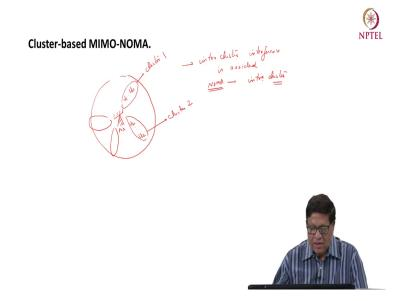
Now, there is also a possibility of cluster based MIMO NOMA. So, in this case what happens suppose the users are spread over in this area and this is for example, the base station here this is antenna. So, these users which are in this area they are actually grouped. So, for example, this could be from U N to U L 1, so this is cluster 1.
