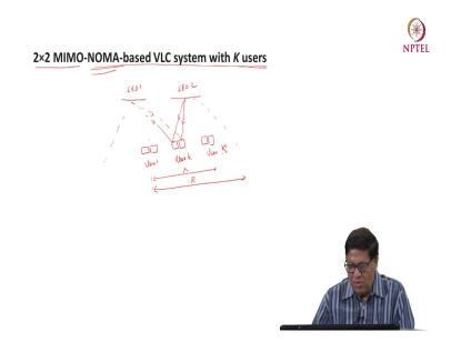
So, let us try to do some calculations using a small example where I am using 2 cross 2 MIMO, NOMA based VLC system and there are K users. So, system diagram is something like this. This is say LED 1, this is say LED 2 and then you have users here and each user has say 2 photodiode. So, be this is a 2 cross 2 MIMO system and similarly here.
