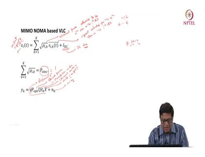
So, the signal x i t this x i t is input signal to the LED input signal to LED 1 or 2 LED i. So, this i can be 1 or 2 in our case is equal to rho i k and this rho i k is actually the electrical power allocated to the kth user in the ith LED. So, rho i k is electrical power allocated to the kth user in the ith LED and this is x i is the input signal to LED i where i is equal to 1 and 2
