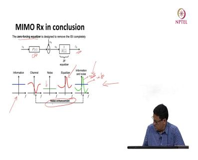
So, in conclusion, MIMO receiver for 0 forcing equalizer; so, this is your channel here, this is the equalizer and this is the estimated output, this is given the information part and this is the channel which is tending going to 0. And if you see the equalizer this thing, this will blow up to infinity because this is 0 forcing receiver.
