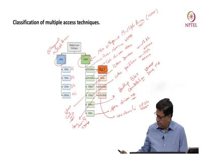
Now, there are various multiple access techniques both in orthogonal space as well as non-orthogonal space. So, this is orthogonal multiple access OMA, OMA Orthogonal Multiple Access. Under this you have FDMA Frequency Division Multiple Access basically 1G system was around this, then TDMA the 2G system was around this and then CDMA 3G system was around this technology and then 4G uses OFDM or optical sorry, Orthogonal Frequency Division Multiple Access.
