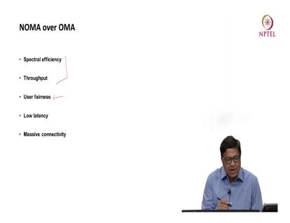
So, these are some of the advantages of NOMA over OMA as we know spectral efficiency and throughput, they are better in NOMA. Because in NOMA users have all the resources irrespective of whether the it has a poor channel condition or a strong channel condition each user actually has all the resources available to available to them.
