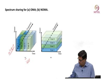
So, this is the basic difference between OMA and NOMA. In OMA you have resources or rb's resource blocks allocated to the users. And this is how this is shown here in this diagram a where frequency resource block is elevated to different users. And in NOMA all the resource block are given to the user and the users have different power levels, but they have all the resource blocks.
