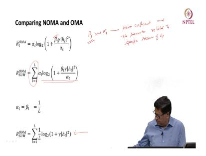
Now, let us start comparing NOMA and OMA. So, for OMA there is Orthogonal Multiple Access. The rate is given by alpha 1 log 2 1 plus beta 1 gamma mod h 1 square divided by alpha 1, where beta 1 and alpha 1 are power coefficient, beta 1 is actually power coefficient. And the and alpha 1 is the parameter related to specific resource of U 1 lth user.
