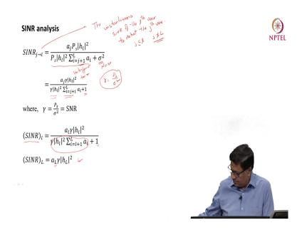
Now, let us do the SINR analysis. So, SINR j to 1 actually this is the instantaneous SINR of the lth user to detect the jth user and j is less than 1 and j is not equal to L. This can be written
