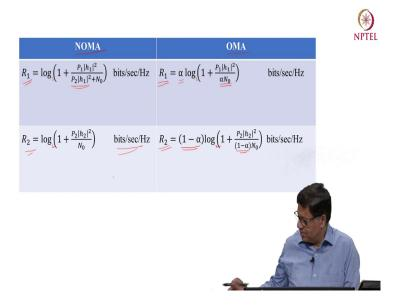
So, just to briefly compare this OMA scheme and NOMA scheme in OMA scheme. So, this is NOMA the R 1 rate user 1 this is for two users. Is this is log to the base 2 everywhere is given by 1 plus P 1 h 1 square P 2 h 1 mod square plus N naught because this is the interference and this is the signal of the user 1.
