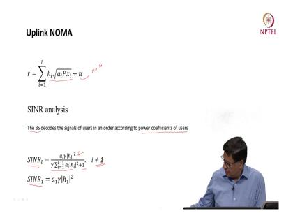
If you see the r, the seed signal is summation coming from different users, h i root a i into P x i plus noise. P is the power, a i is the power coefficient, P is the total power which is scaled down scaled by power coefficient factor a i. So, doing SINR analysis, the base station decodes the signals of users in an order according to the power coefficient of the users.
