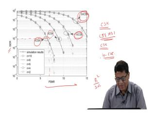
And if I plot those curves because that integral is difficult to solve so, you have to solve it numerically and this is a result for different CSK. This is 4CSK, 8CSK, 16CSK, and 64CSK and these are the simulation and analytical results. So, the dashed lines are analytical results and the hard lines are sim simulation results.
