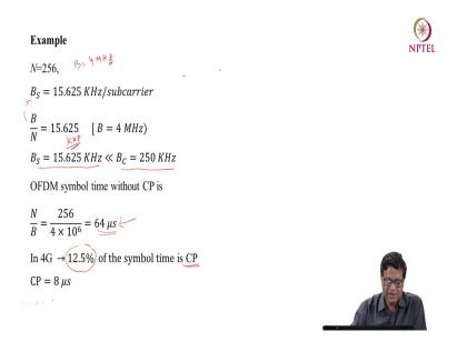
So, B by N will be 4 megahertz divided by N will give you 15.6 kilohertz. So, this is per subcarrier this is what I have written here. So, this becomes your B by N. So, if you see this B S and your B S for a wireless N is 250 kilohertz this B s is much less than B C. So, OFDM symbol time without cyclic prefix will be N by B this is symbol time N is equal to 256 and B here bandwidth is 64 micro second.
