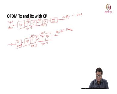
So, now we are in a position to draw the complete diagram of OFDM transmitter in receiver. So, this is your input stream. First operation what we do is serial to parallel. So, you get this different data x 0 to x minus 1 and then we do IFFT. This is quite common IDFT algorithm IFFT endpoint and then you get these symbols here.
