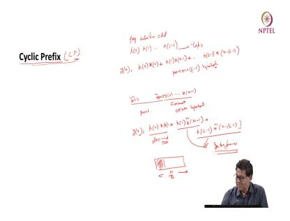
Hello everyone. So, now we will introduce the idea of Cyclic Prefix or CP. So, any frequency selective channel can be modelled as using channel taps or like h 0, h 1 or h, L minus 1, say upto lth. So, this is any frequency selective channel and these are the taps. So, what happens because of this channel? If you see any signal at time stand n y n then it will be h 0, x n and x h 1, x n minus 1 plus so on and 00730, forth and the last one is h 1 minus 1, x n minus L minus 1.
