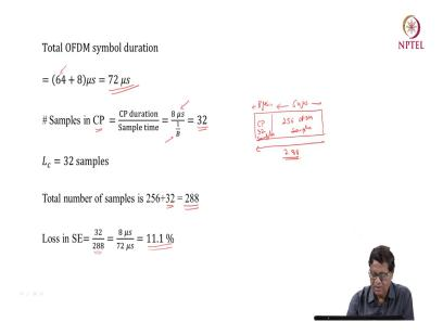
So, the total OFDM symbol duration which will be CP and the 64 which has come earlier. Let us see this 64 is N by B OFDM symbol time without C P. So, this is without C P with C P is 8. So, this is the total OFDM symbol duration which is 72 micro second. And number of samples if you see in C P the C P duration is 8 micro second this is we have seen earlier slides and sample time is 1 by B.
