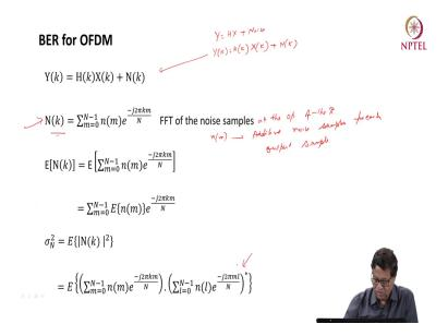
Now, let us try to calculate the BER for OFDM. Bitter a rate for OFDM the we had calculated for baseband. So, we will also calculate for OFDM. So, right now it is nothing to do with optical wireless channel right now I am discussing about the fundamentals of OFDM and how it behaves in RF channel.
