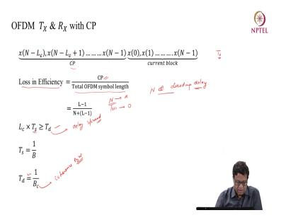
So, now let us understand OFDM transmitter and RX with CP. How normally it is done? So, this is your current block x 0 to x N minus 1. These are the samples and depending upon the delay spread T d you select those samples and prefix it in the middle in the beginning. So, this is what is the CP and I have selected L C number which are prefixed. So, this becomes OFDM symbol complete OFDM symbol. And because of this addition of CP there is a loss in efficiency.
