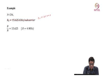
So, let us understand an example if N is equal to 256 that is the number of subcarriers and B s is say 15.625 kilohertz per subcarrier. So, B by N this is B this is actually B this is; B this is not correct. So, B is 15.625 kilohertz. So, B by N or I am sorry. So, this is your B is 4 megahertz.
