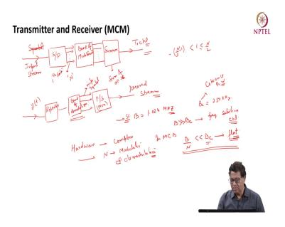
Now, let us draw a diagram for this multi carrier modulation what does it look like. So, this is your symbol. The first operation you do is yours do the serial to parallel conversion and then you get different outputs that is the different data different data for example, this is you know serial data x i x i plus 1 and so on so forth.
