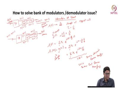
So, let us try to understand this and this was solved by two engineers Weinstein and Ebert. So, what they did that your s t signal has bandwidth B. Now, if I sample this this system this signal at Nyquist rate sample at Nyquist rate which is say t s given by 1 by B that is a radii simple sample at. So, I get a Uth sample which is at instant UT s this is the Uth sample at UT s this is a s i T.
