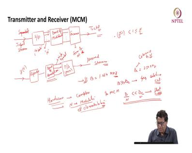
Because the bandwidth B by N the sub band bandwidth is much less than the B c and so, you are able to recover your data signal. So, how to solve this problem of hardware complex hardware how to get rid of this so many modulators and demodulators which makes your circuit very complex.
